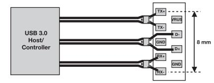
Three TPD2EUSB30 to protect USB 3.0 Class A connector (requires only one layer of routing).
