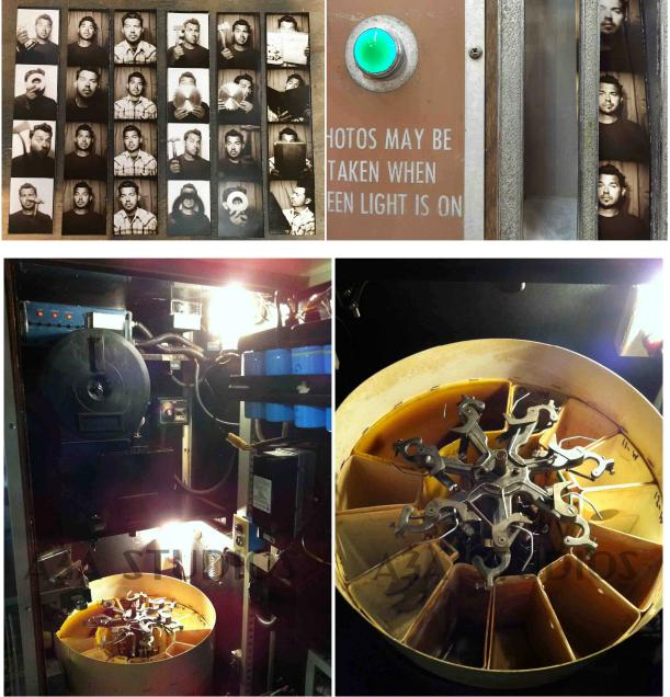
Inside a Vintage Model-21 Photo-Me AP10 System Photobooth (showing tanks, arms, spider assembly, plate camera & paper magazine)
