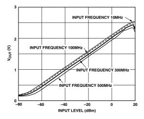
Figure 8. AD8307 Log Transfer Function
