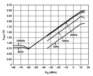
Figure 41. AD8362 Transfer Function for  $C_C = 10 \ \mu F$
