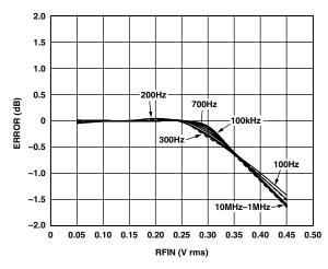
Figure 35. AD8361 Law Conformance for  $C_C = 10 \ \mu F$
