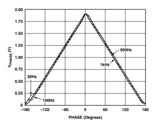
Figure 55. AD8302 Phase Output for  $C_C = 100 \ \mu F$
