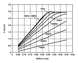
Figure 31. AD8361 Transfer Function for  $C_C = 1 \ \mu F$
