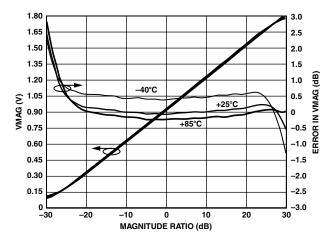
Figure 47. AD8302 Log Slope and Error at 100 MHz
