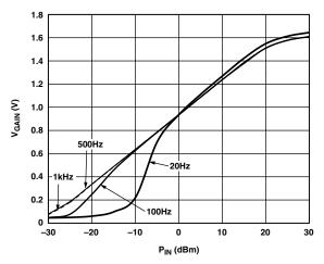
Figure 54. AD8302 Gain Output for  $C_C = 100 \ \mu F$
