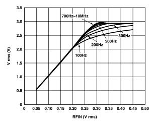
Figure 33. AD8361 Transfer Function for  $C_C = 100 \ \mu F$
