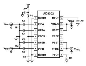
Figure 46. AD8302 Basic Connections
