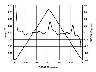
Figure 52. AD8302 Phase Output and Conformance at 10 kHz for  $C_c = 1 \ \mu F$
