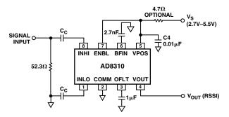
Figure 27. AD8310 Modifications for Low Frequency Operation
