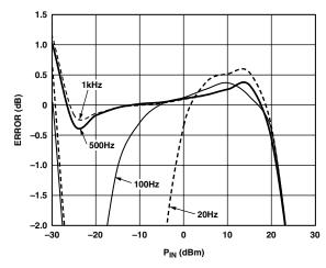
Figure 56. AD8302 Gain Conformance for  $C_C = 100 \ \mu F$
