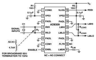
Figure 17. AD8309 Basic Connections
