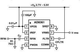
Figure 28. AD8361 Basic Connections
