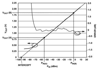
Figure 1. Basic Log Amp Transfer Function
