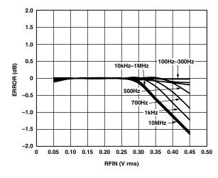
Figure 34. AD8361 Law Conformance for  $C_C = 1 \ \mu F$
