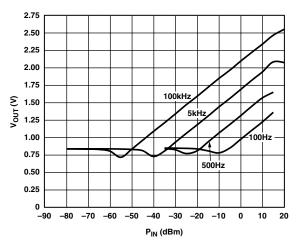
Figure 11. AD8307 Transfer Function for  $C_C = 0.1 \ \mu F$
