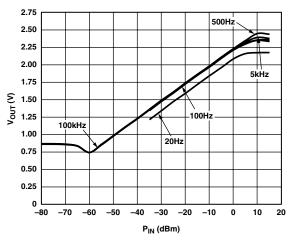
Figure 42. AD8362 Transfer Function for  $C_C = 100 \ \mu F$
