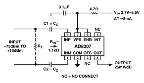
Figure 7. AD8307 Basic Connections
