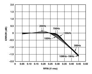
Figure 36. AD8361 Law Conformance for  $C_C = 100 \ \mu F$
