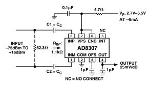
Figure 10. AD8307 Modifications for Low Frequency Operation
