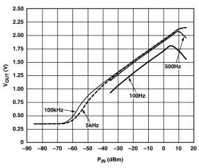
Figure 5. AD8306 Detector Transfer Function for Low Frequencies
