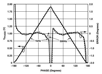
Figure 53. AD8302 Phase Output and Conformance for  $C_c$  = 4.7  $\mu$ F
