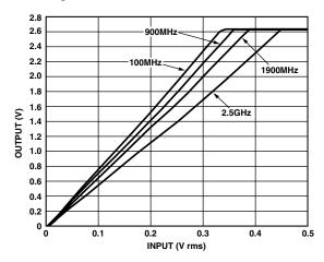
Figure 29. AD8361 Slope at Various Frequencies, GND Reference Mode, 2.7 V Supply
