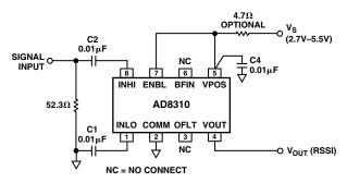
Figure 22. AD8310 Basic Connections
