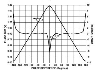
Figure 48. AD8302 Phase Output and Nonlinearity
