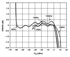
Figure 45. AD8362 Law Conformance for  $C_C = 100 \ \mu F$
