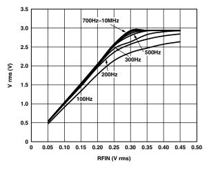
Figure 32. AD8361 Transfer Function for  $C_C = 10 \ \mu F$
