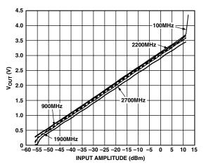
Figure 38. AD8362 Log Slope for Various Frequencies
