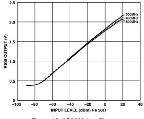
Figure 18. AD8309 Log Slope
