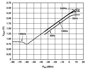
Figure 13. AD8307 Transfer Function for  $C_C = 100 \,\mu F$
