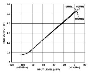
Figure 23. AD8310 Log Slope
