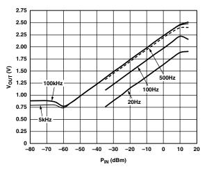
Figure 12. AD8307 Transfer Function for  $C_C = 10 \ \mu F$
