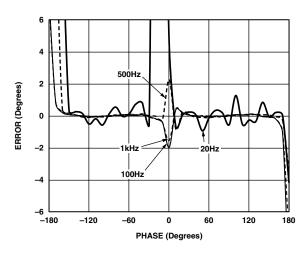
Figure 57. AD8302 Phase Conformance for  $C_{C}$  = 100  $\mu$ F
