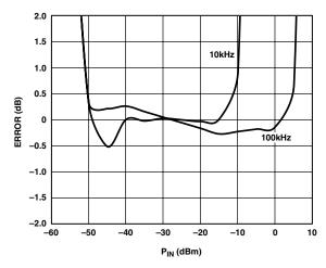
Figure 43. AD8362 Law Conformance for  $C_C = 0.1 \ \mu F$
