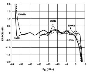
Figure 44. AD8362 Law Conformance for  $C_C = 10 \ \mu F$
