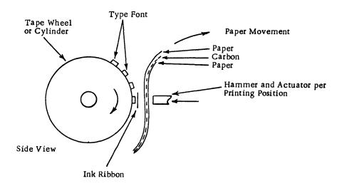
Figure 2-24 Rotating Drum Printer
