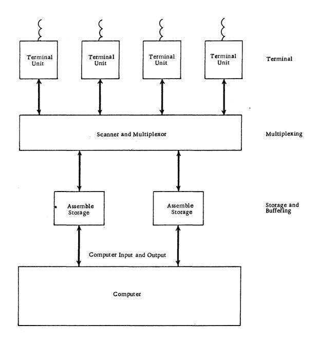
Figure 2-34 Schematic of Typical Interface Functions in Digital Machineto-Machine Communication
