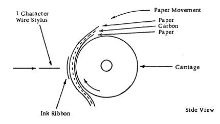
Figure 2-27 Stylus Printer
