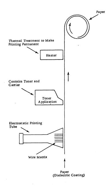
Figure 2-31 Electrographic Printer
