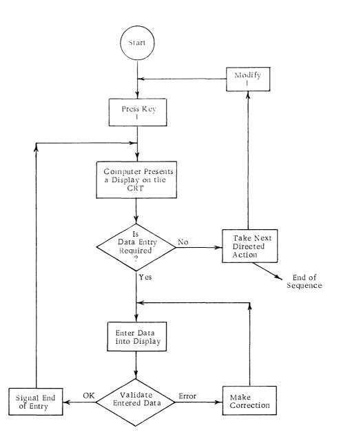
Figure 2-10 Typical Operator Steps in Use of Function Keys
