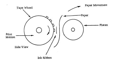
Figure 2-25 Impact Wheel Printer
