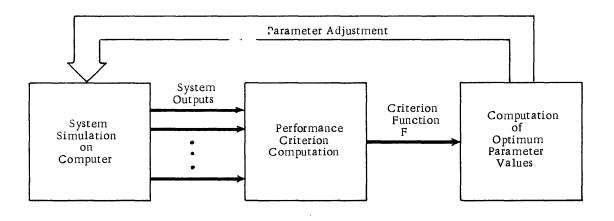
Figure 3-5, Block Diagram of Design Optimization Problem
