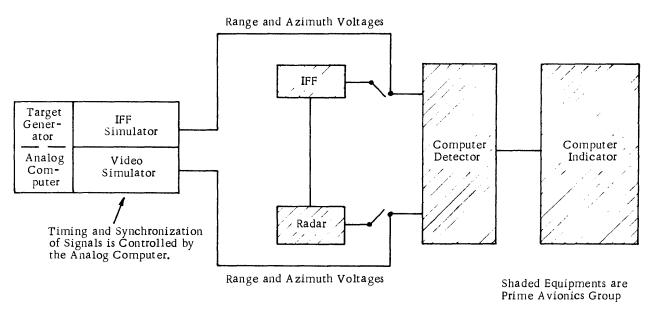
Figure 3-11 Radar Data Input Simulation
