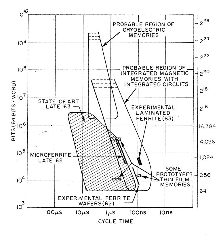
Figure 2-35 - Storage Capacity and Cycle Time of Memories (After Rajchman)
