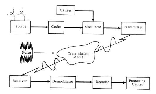
Figure 3-6, Carrier Transmission System
