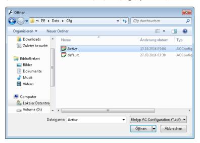
If the user wishes to make changes to or expand an existing configuration to be activated at a later date, then s/he can open a basic configuration, modify it and then save it under a different name. In this way it is possible to re-use and expand upon previous configurations, and one does not have to start every time from the very basic settings in **default.acf.**
