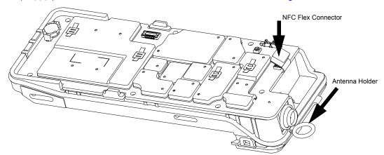
Figure 8-17. Assemble the Main O-Ring at Antenna Holder
