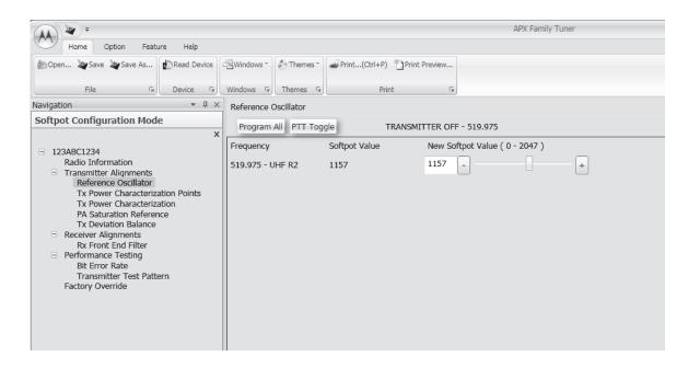
Figure 6-6. Reference Oscillator Alignment Screen (UHF2)
