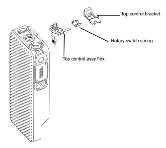
Figure 8-15. Serviceable Components – Main Housing
