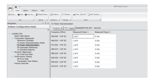
Figure 6-14. Transmit Power Characterization Alignment Screen (UHF2)
