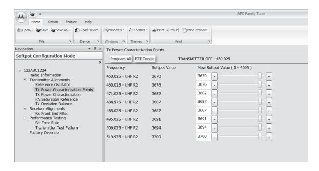
Figure 6-10. Transmit Power Characterization Points Alignment Screen (UHF2)
