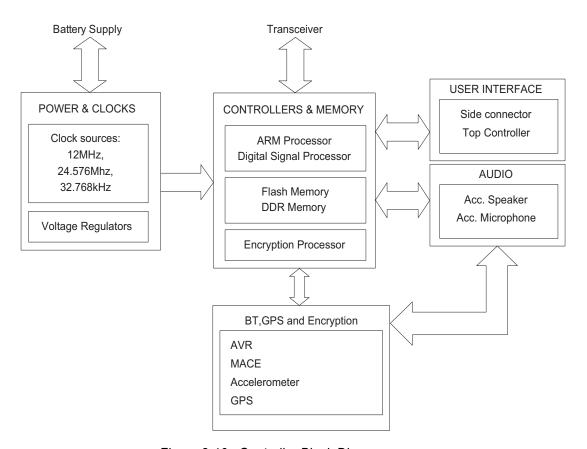
Figure 3-10. Controller Block Diagram
