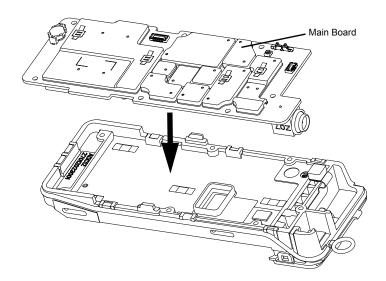
Figure 8-18. Assemble the RF Board
