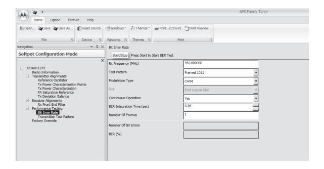
Figure 6-28. Bit Error Rate Screen (UHF2)
