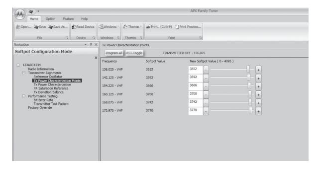
Figure 6-11. Transmit Power Characterization Points Alignment Screen (VHF)
