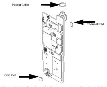
Figure 8-13. Serviceable Components - Main Board Assembly
