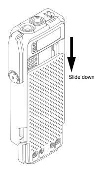
Figure 8-5. Removing the Battery
