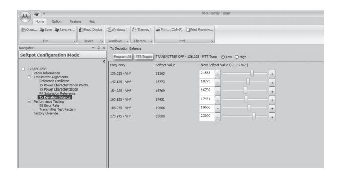
Figure 6-23. Transmit Deviation Balance Alignment Screen (VHF)
