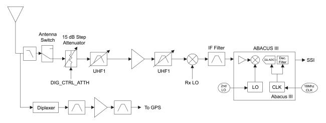
Figure 3-2. Receiver Block Diagram (UHF1)
