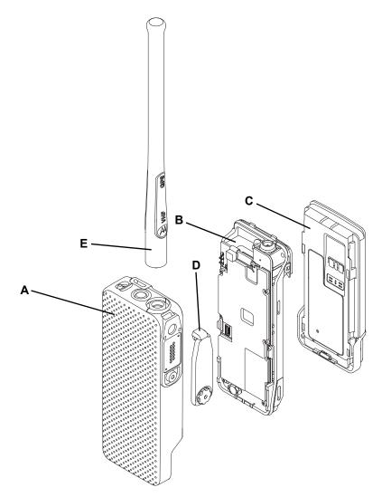
Figure 8-1. APX 3000 Partial Exploded View
