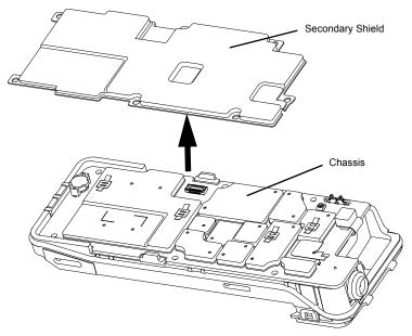
Figure 8-9. Remove the Secondary Shield Assembly
