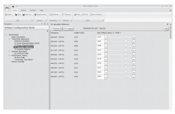
Figure 6-17. PA Saturation Referencing Alignment Screen (UHF1)
