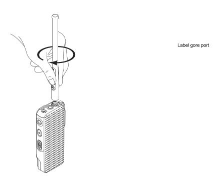
Figure 8-25. Attaching the Antenna
