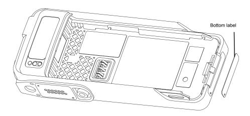
Figure 8-28. Assemble the Bottom Label
