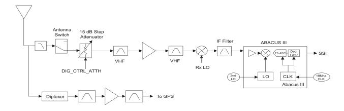
Figure 3-4. Receiver Block Diagram (VHF)
