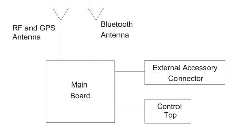
Figure 3-1. APX 3000 Overall Block Diagram
