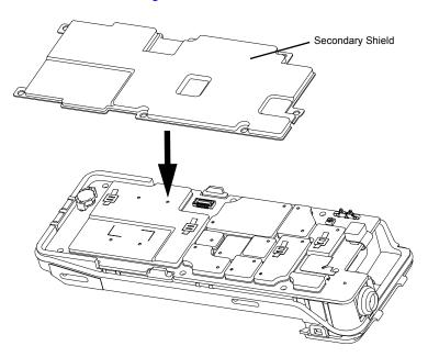
Figure 8-19. Assemble the Secondary Shield Assembly
