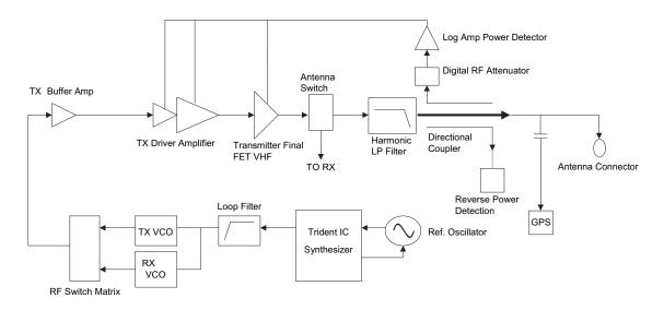
Figure 3-8. Transmitter (VHF) Block Diagram
