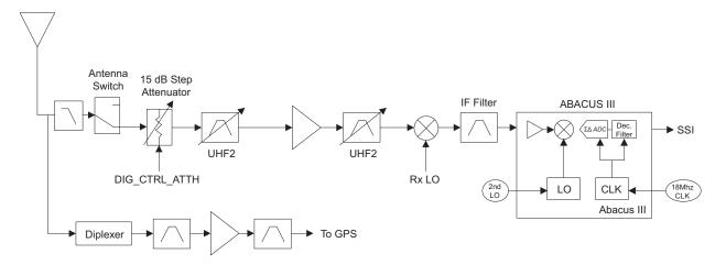
Figure 3-3. Receiver Block Diagram (UHF2)
