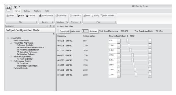
Figure 6-26. Front End Filter Alignment Screen (UHF2)
