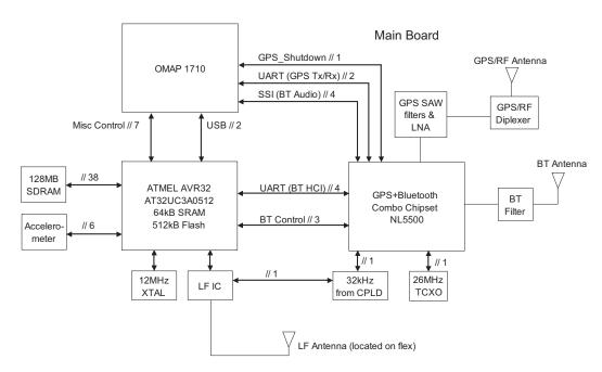
Figure 3-11. GPS/Bluetooth/Accelerometer Block Diagram
