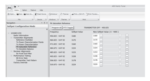
Figure 6-18. PA Saturation Referencing Alignment Screen (UHF2)
