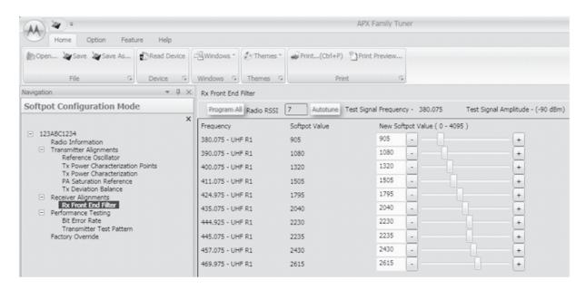
Figure 6-25. Front End Filter Alignment Screen (UHF1)
