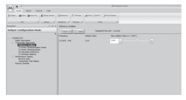
Figure 6-7. Reference Oscillator Alignment Screen (VHF)
