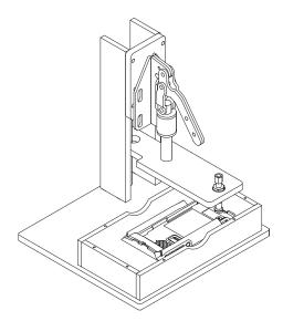
Figure 8-30. Attaching Vacuum Test Fixture
