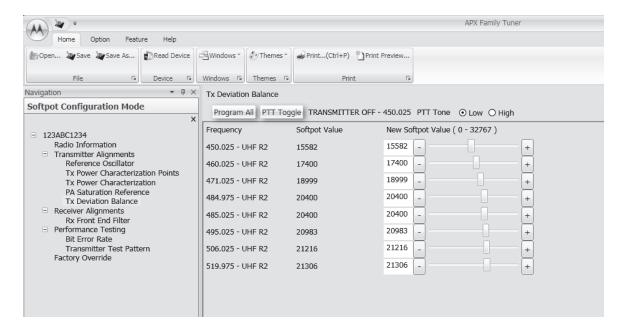
Figure 6-22. Transmit Deviation Balance Alignment Screen (UHF2)
