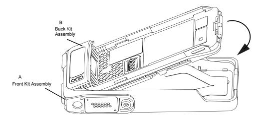
Figure 8-22. Assemble Back Kit and Front Kit together
