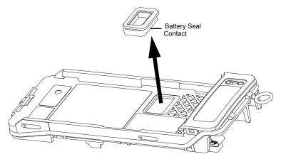
Figure 8-12. Remove Battery Seal
