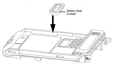
Figure 8-16. Assemble the Battery Seal
