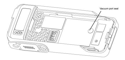
Figure 8-26. Assemble the Seal, Vacuum Port
