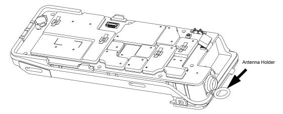
Figure 8-10. Remove the Main O-Ring at the antenna holder
