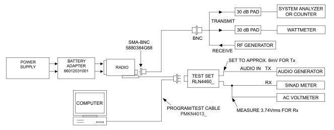
Figure 6-1. Radio Alignment Test Setup
