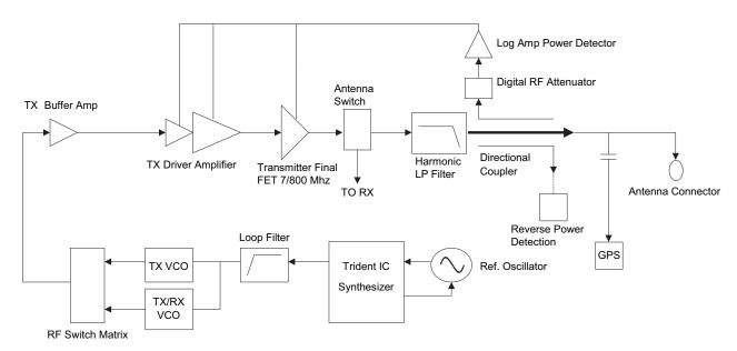
Figure 3-9. Transmitter (700/800 MHz) Block Diagram
