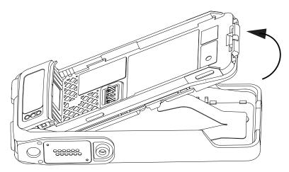
Figure 8-7. Remove the Chassis Assembly
