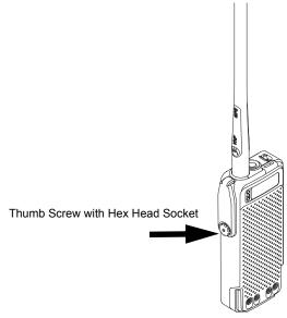
Figure 8-2. Removing the Thumb Screw
