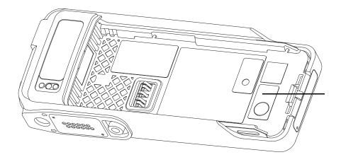
Figure 8-27. Assemble the Label Gore Port
