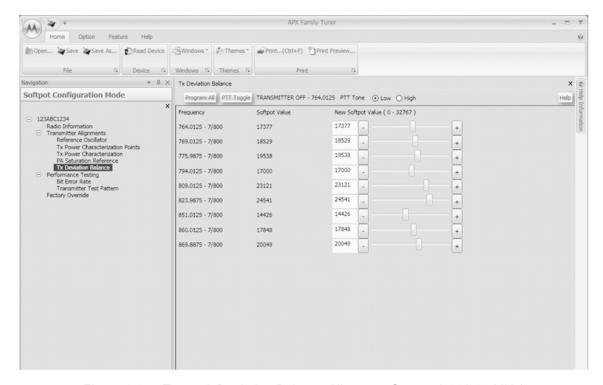
Figure 6-24. Transmit Deviation Balance Alignment Screen (700/800 MHz)
