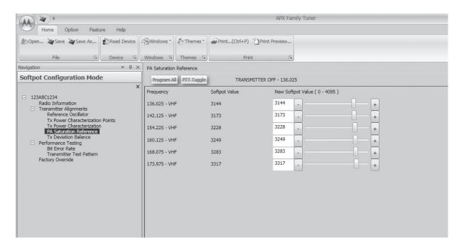
Figure 6-19. PA Saturation Referencing Alignment Screen (VHF)
