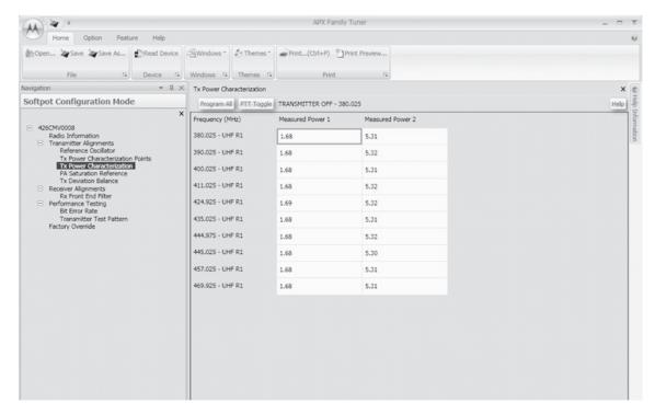
Figure 6-13. Transmit Power Characterization Alignment Screen (UHF1)
