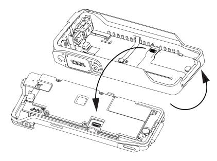
Figure 8-21. Slide chassis assembly into Front Housing
