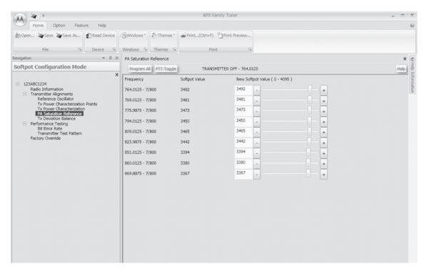
Figure 6-20. PA Saturation Referencing Alignment Screen (700/800 MHz)
