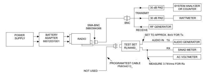
Figure 5-1. Performance Checks Test Setup
