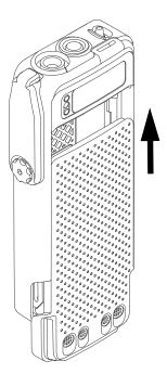
Figure 8-29. Attaching Battery – Slide into Position
