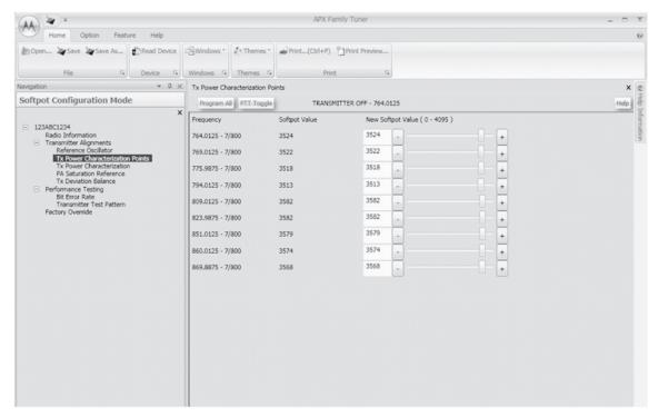
Figure 6-12. Transmit Power Characterization Points Alignment Screen (700/800MHz)
