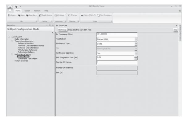
Figure 6-30. Bit Error Rate Screen (700/800 MHz)
