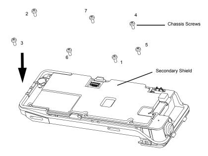
Figure 8-20. Torque in the Chassis Screws.
