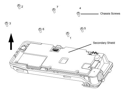
Figure 8-8. Remove the chassis screws
