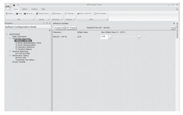
Figure 6-5. Reference Oscillator Alignment Screen (UHF1)
