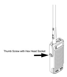
Figure 8-24. Securing the Cover
