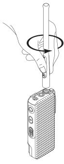
Figure 8-3. Removing the Antenna
