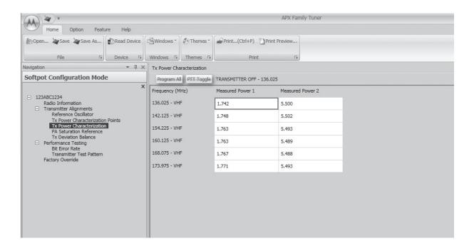
Figure 6-15. Transmit Power Characterization Alignment Screen (VHF)
