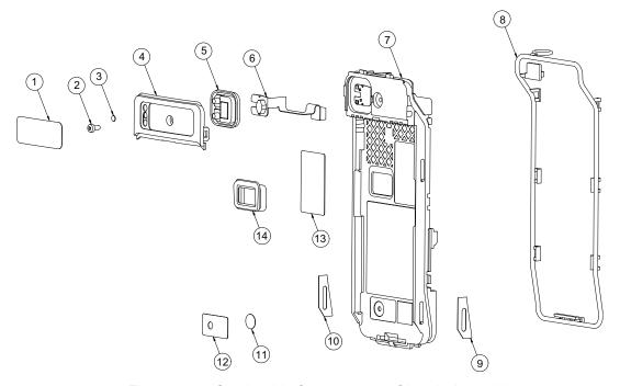
Figure 8-14. Serviceable Components - Chassis Assembly
