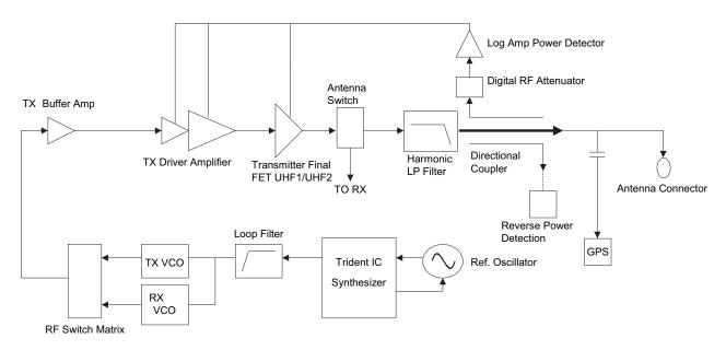
Figure 3-7. Transmitter (UHF1/UHF2) Block Diagram
