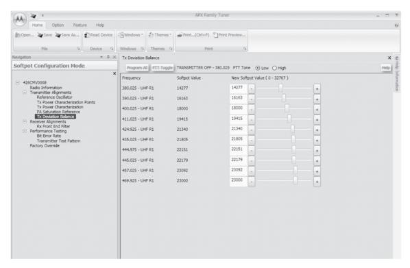
Figure 6-21. Transmit Deviation Balance Alignment Screen (UHF1)
