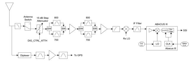
Figure 3-5. Receiver Block Diagram (700/800 MHz)
