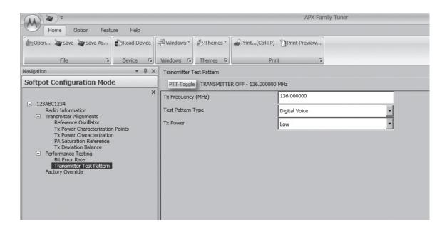
Figure 6-33. Transmitter Test Pattern Screen (VHF)
