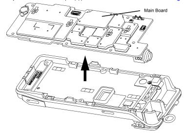
Figure 8-11. Lift up the Main Board from the Chassis
