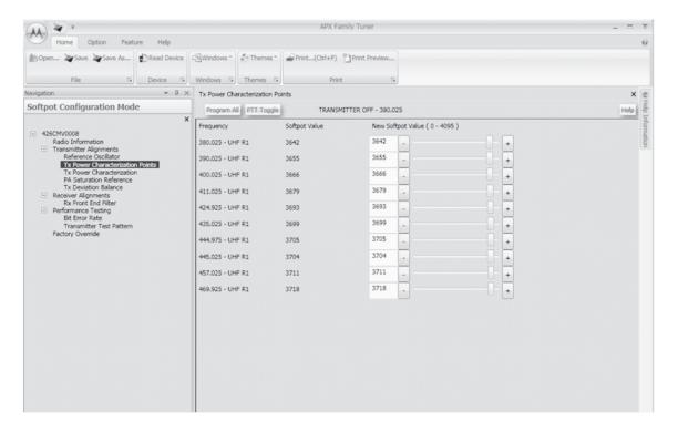
Figure 6-9. Transmit Power Characterization Points Alignment Screen (UHF1)
