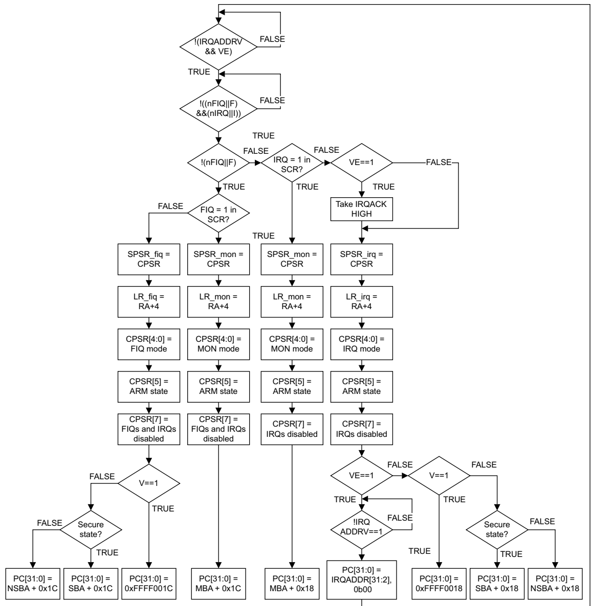
Figure 12-3 Interrupt entry sequence
