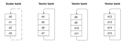
Figure C5-2 Double-precision register banks
