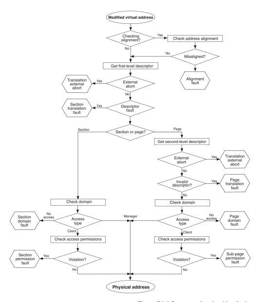
Figure B4-2 Sequence for checking faults
