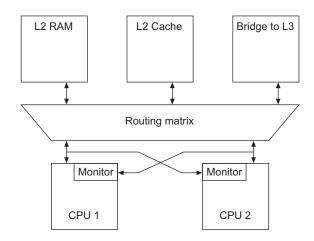
Figure A2-3 Write snoop monitor approach
