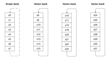
Figure C5-1 Single-precision register banks
