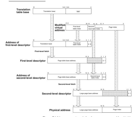
Figure B4-6 Large page translation in a coarse second-level table
