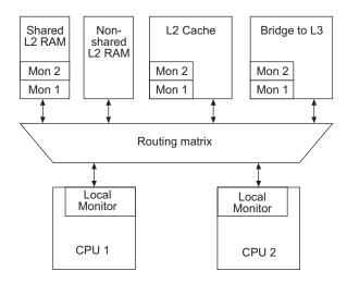
Figure A2-4 Monitor-at-target approach
