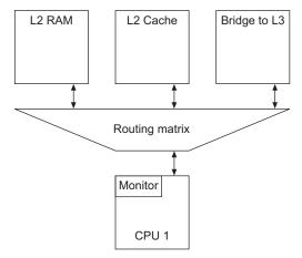
Figure A2-2 Example uniprocessor (non-shared) monitor
