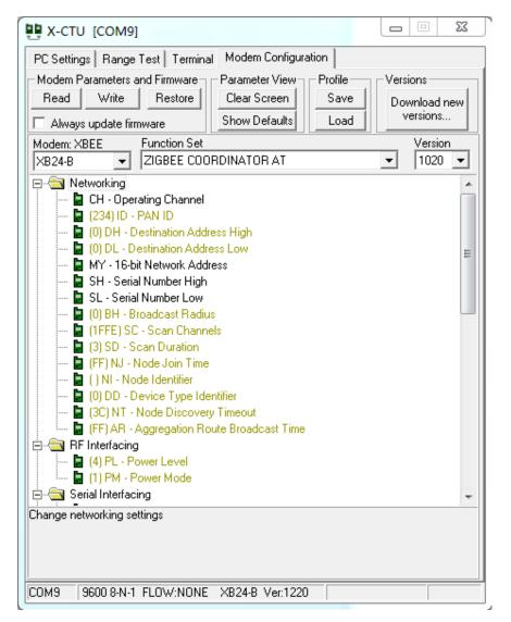
Figure 10: Reading out current parameters
