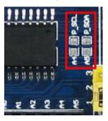
Figure 22: Setting the pins A4 and A5 as I2C control pins
