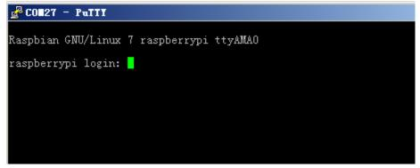
Figure 4: Connecting PuTTY to Raspberry Pi board
