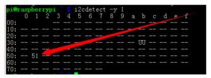
Figure 17: The device address of PCF8563 connected to Raspberry Pi
