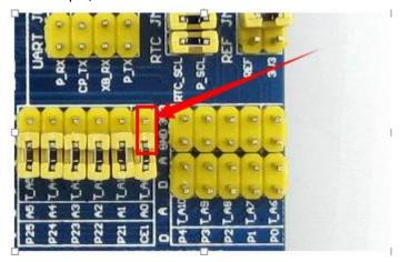
Figure 19: connecting Pin T\_A0 to Pin A0
