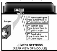
Remote Car Starters of this series are equipped with an on-board high-current programmable 5<sup>th</sup> Relay that can be used to power a second Ignition, Accessory or Crank wire.
