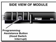
(A.k.a. the **PAB**.) Mounted on the Remote Car Starter, this button can be used from within the vehicle instead of the Hood Pin switch in the Engine compartment. This will spare the installer the trouble of accessing the Hood Pin switch in the Engine compartment.
