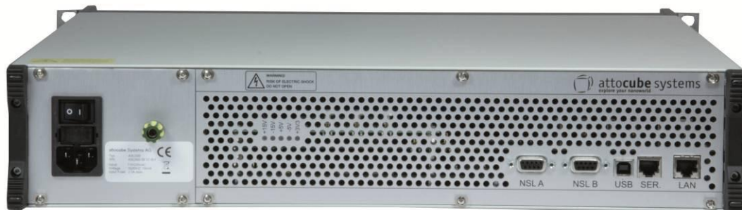
Figure 5: Back panel of the ASC500 v2. Please note the new digital interface (NSL) and the LAN connection.
