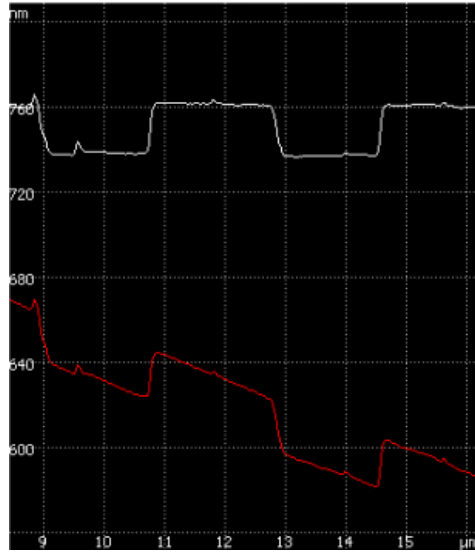
Figure 17: A typical line scan before (red) and after (white) the sample tilt is compensated by the Slope Compensation feature.
