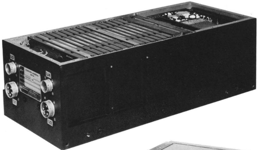
AN/APN 131 COMPUTER — This computer, used in the F105, is the predecessor of the current MINAC series and pioneered many of the advanced concepts incorporated in the later computers designed by the company. Looking to the future, new analog, digital, and hybrid computers are being designed for advanced applications in manned aircraft and space vehicles.
