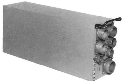
GPK-20 COMPUTER — A general-purpose digital computer for navigation and weapons delivery in military aircraft. Has modular random-access solid-state expandable core memory, arithmetic and control sections, A/D conversion, and power supply in a single unit, and incorporates self-protection against memory loss.
