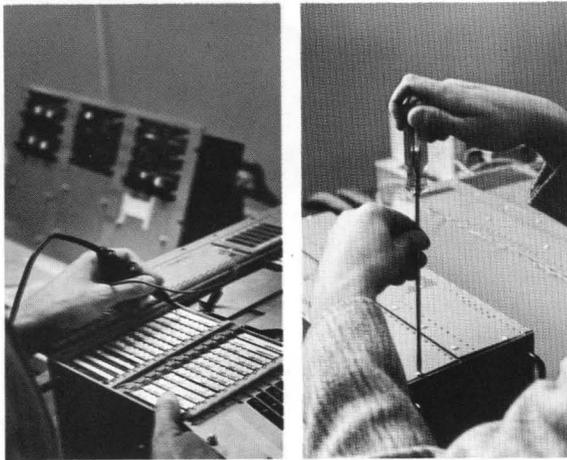
*The AN/ASN-24 (G) was designed for exceptionally simple testing, service, and repair. Accurate, uncomplicated test equipment and procedures help to speed check-out and fault isolation. Modular "building-block" construction helps to facilitate the replacement of defective units.*
