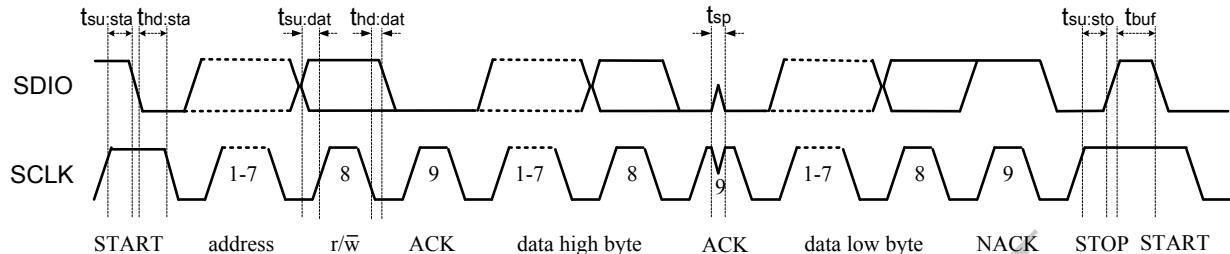
Figure 2. I<sup>2</sup>C Interface Read Timing Diagram
