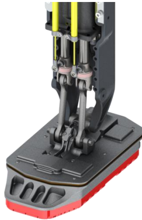
Figure 6: Ankle joint featuring a coupled transmission between two actuators and two intersecting joints
