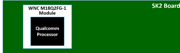
Figure (Appendix) 4 - SK2 Nested Processor Modules
