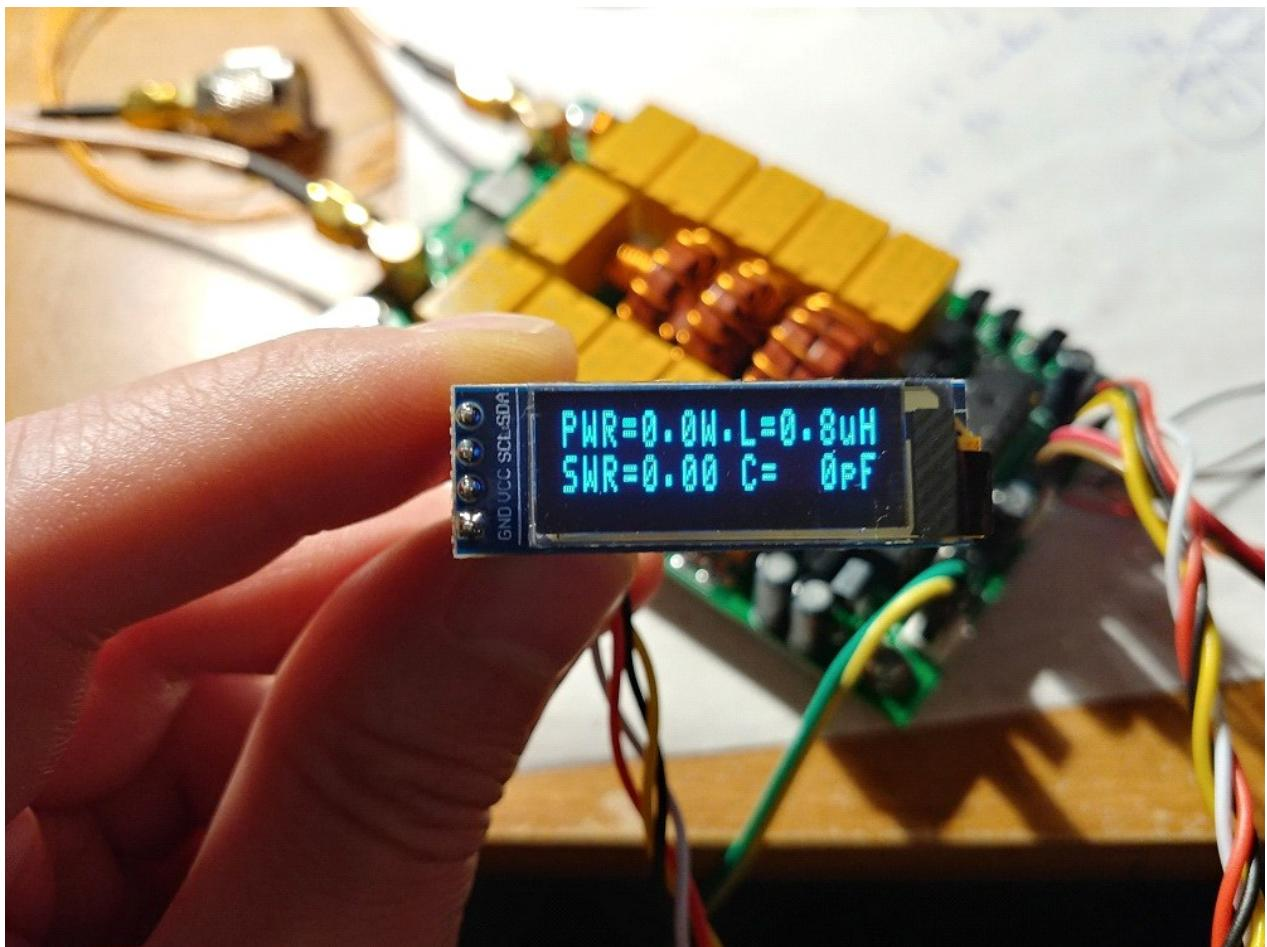
The indication on the 0.91 128x32 display looks like on a regular 1602 display, while having tiny dimensions.
