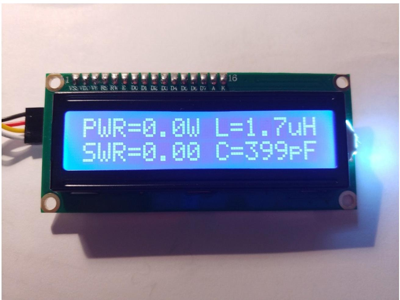
The left side of the indicator displays the power throughput and SWR. The peak detector mode is used, which allows to accurately measure the signal power of the transmitter when using various types of modulation.
