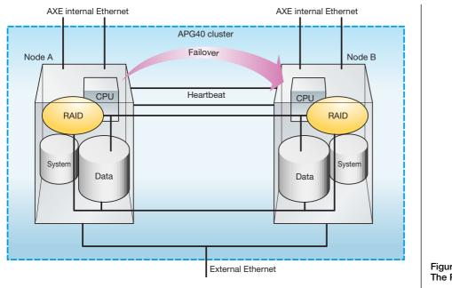
Figure 13 The RAID hardware system.
