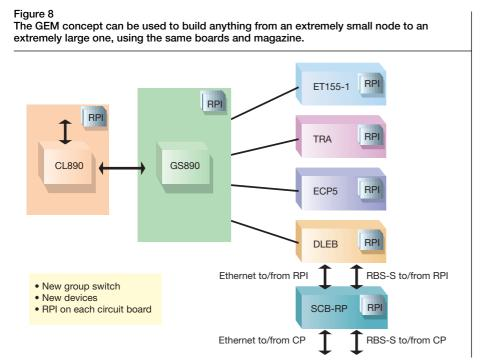
advances in technology to modify the architecture rather than merely shrink the hardware. One advantage of this change is that considerably fewer magazine and board types are needed in each node. A second advantage is that many internal AXE interfaces have been moved to the GEM backplane, reducing the need for cables. As shown in Figure 7, many different functions can be mixed in the GEM.
