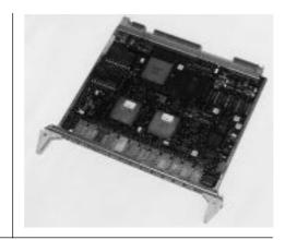
Photograph of the switch distributed board (XDB).
