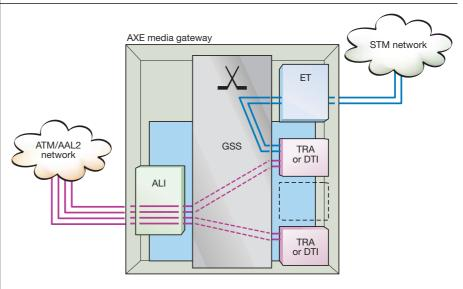
Switched 64 kbit/s connections for PCM coded voice
