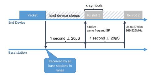
The End-device, e.g. a temperature sensor, wakes-up to transmit its measurement. The LoRaWAN radio frame will be received by all nearby base stations of the RF network. The device then immediately goes to sleep for a specified amount of time, by default 1 second, in order to preserve the battery.
