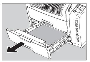
If a film is jammed, gently remove the sheet. Reposition the film stack in the film tray, making sure that all the sheets are kept correctly (refer to *Loading films*' on page 44).
