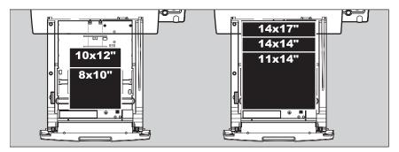
Appropriate labels have been applied on the input tray(s) by the service personnel at installation of the printer, indicating the type of new film to be loaded when the tray is empty.
