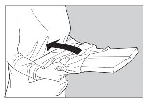
7 Slide the film pack into the input tray, and remove the plastic film bag completely.
