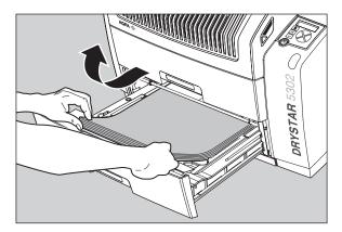
**3** Check if the film feed section of the input tray is clear.
