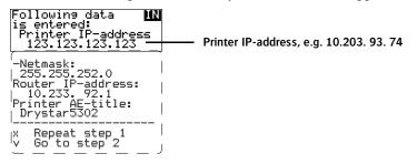
**11** Press the Confirm key to go to step 2 of the installation wizard or press the Escape key to repeat step 1.
