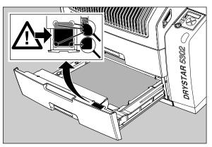
When the tray is closed, the Film Identification tag is read and the printer settings are automatically adjusted if the film properties have changed. The Film Identification tag is located on the protective sheet on the backside of the film pack. The figure below shows the film pack upside down.
