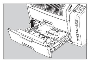
4 Locate the correct tab position for the desired film format.
