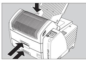
Film transport jams (clearing from the top section)
