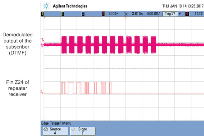
Figure 7: Oscilloscope showing DTMF output on Pin Z24 (Bad Tune)
