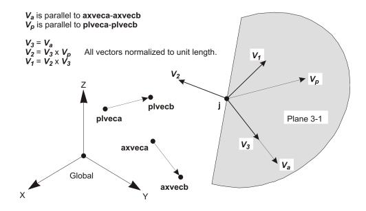
**Figure 56**Example of the Determination of the Solid Element Local Coordinate System Using Reference Vectors for **local**=31. Point **j** is the Center of the Element.
