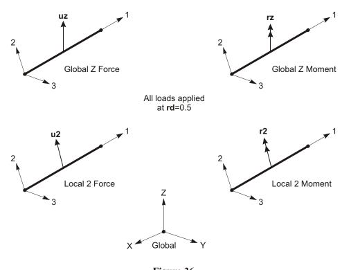
**Figure 36** *Examples of the Definition of Concentrated Span Loads*
