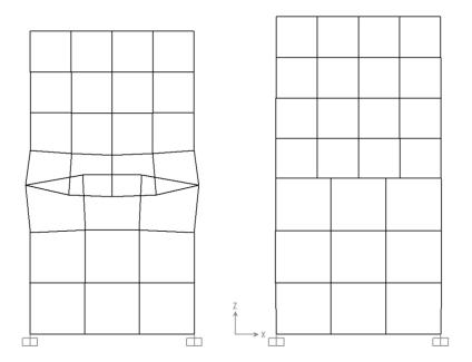
**Figure 44**Connecting Meshes with the Edge Constraints: Left Model – No Edge Constraints; Right Model – Edge Constraints Assigned to All Elements
