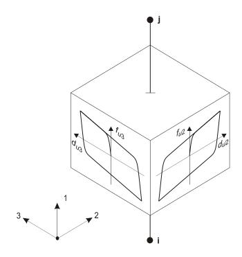
**Figure 73**Hysteretic Isolator Property for Biaxial Shear Deformation
