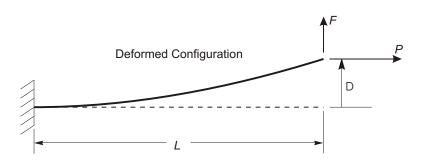
**Figure 84**Geometry for Cantilever Beam Example
