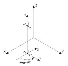
Local 1 Axis is Parallel to +Z Axis Local 2 Axis is Rotated 90° from X-1 Plane
