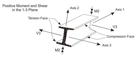
**Figure 39**Frame Element Internal Forces and Moments
