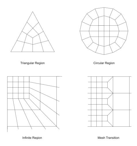
**Figure 43** *Mesh Examples Using the Quadrilateral Area Element*
