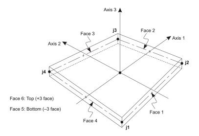
Four-node Quadrilateral Shell Element
