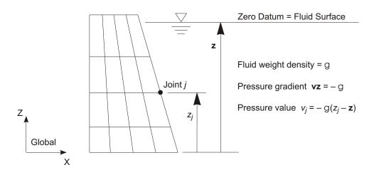
**Figure 79**Example of a Hydrostatic Pressure Pattern
