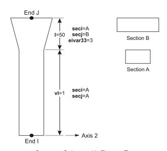
Concrete Column with Flare at Top
