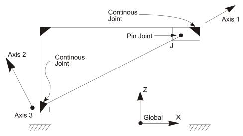
For diagonal element: R3 is released at end J
