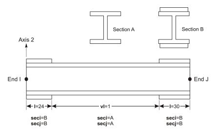
Steel Beam with Cover Plates at Ends
