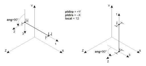
Local 1 Axis is Not Parallel to **pldirp** (+Y) Local 2 Axis is Rotated 90° from Y-1 Plane
