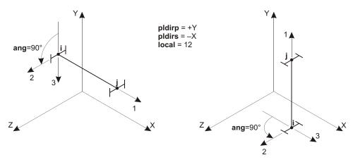
Local 1 Axis is Not Parallel to **pldirp** (+Y) Local 2 Axis is Rotated 90° from Y-1 Plane Local 1 Axis is Parallel to **pldirp** (+Y) Local 2 Axis is Rotated 90° from X-1 Plane
