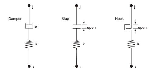
**Figure 67**Maxwell Dampers, Gap, and Hook Property Types,
