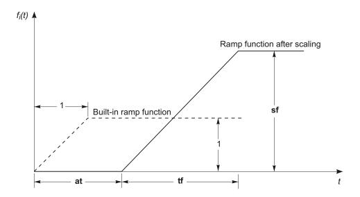
**Figure 83**Built-in Ramp Function before and after Scaling
