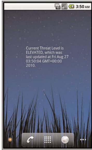
Figure 22.2 A Simple App Widget on the Home screen that displays the security threat level.
