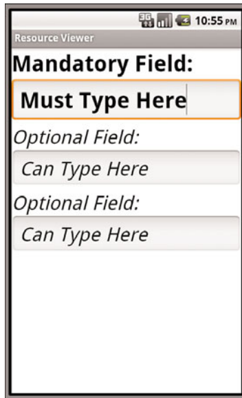
Figure 6.6 A layout using two styles, one for mandatory fields and another for optional fields.
