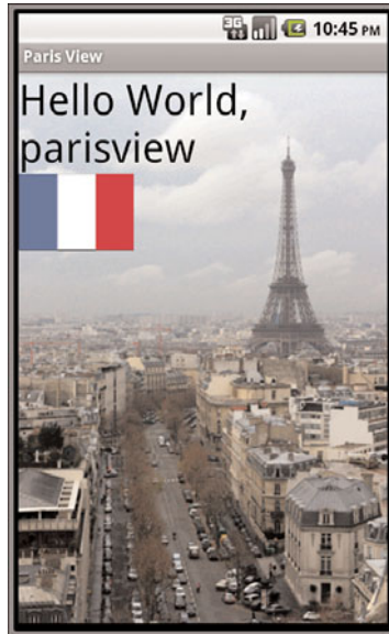
Figure 6.5 A layout with a LinearLayout , TextView , and ImageView , shown in the Android emulator.
