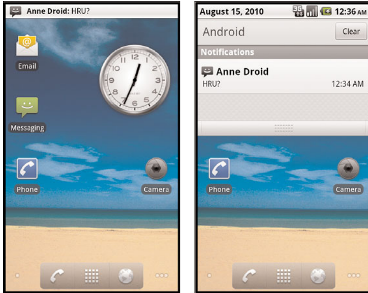
Figure A.13 An incoming SMS from 555-1212 (configured as a contact named Anne Droid), prompted via the emulator console.
