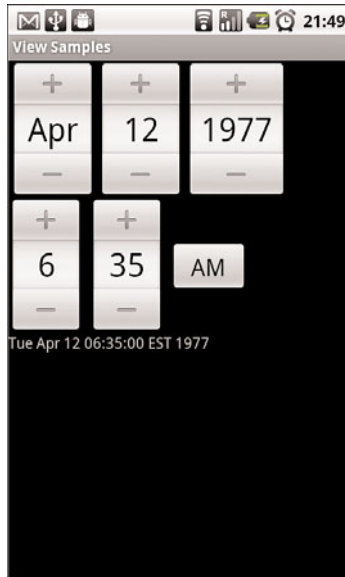
Figure 7.8 Date and time controls.
