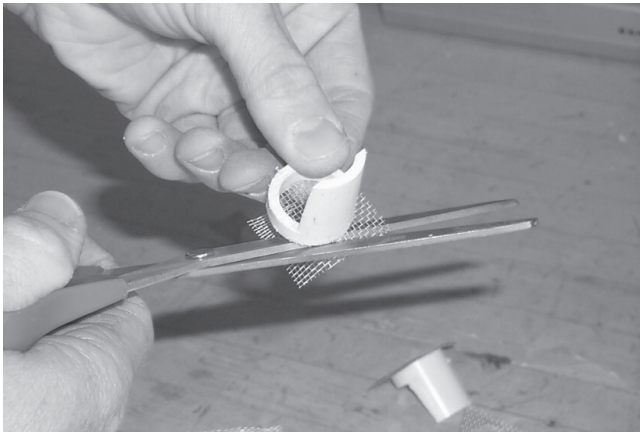
Figure A.4. Cutting out baskets from screen.
