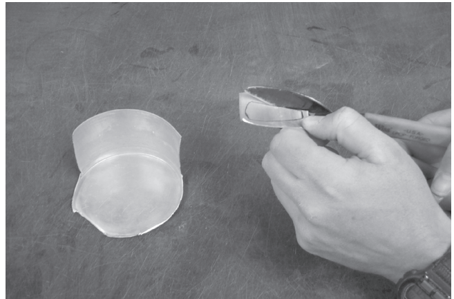
Figure A.5. Cutting shovels with tin snips.
