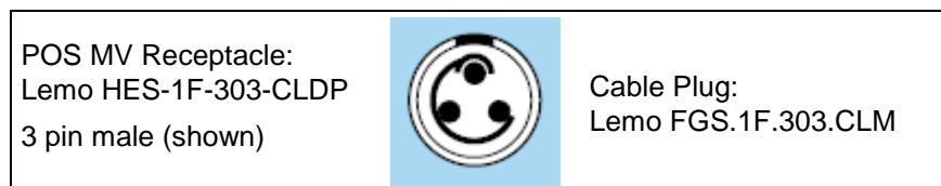
Figure 8: PWR Connector Pin Arrangement
