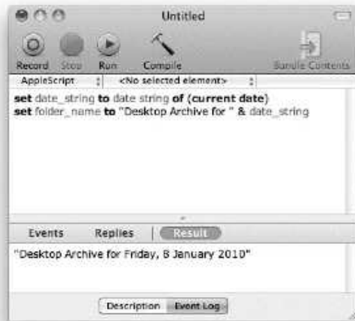
Figure 3–2. The result of running the first two completed lines of the script
