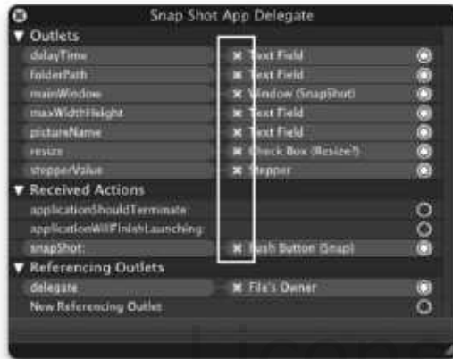
Figure 30–20. Removing connections in Interface Builder
