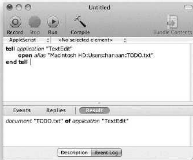
Figure 5–1. Sending an open command to the TextEdit application to open a text file
