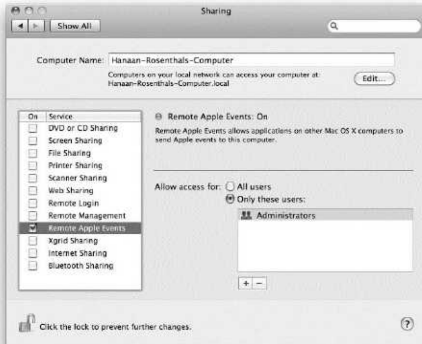
Figure 12–1. The System Preferences Sharing panel, where you turn on remote Apple events
