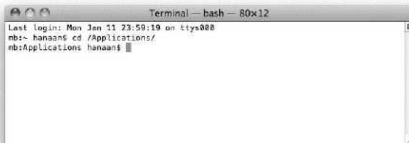
Figure 27-3. The Terminal window shown after the cd command. Watch how the command prompt changes.
