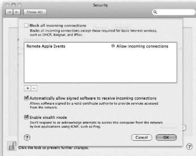
Figure 12–2. The System Preferences Security panel, where you configure the Mac OS X firewall
