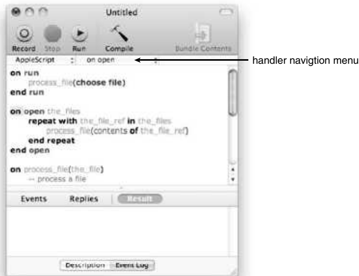
Figure 4–5. The script navigation menu—in this example, the open handler has been chosen.
