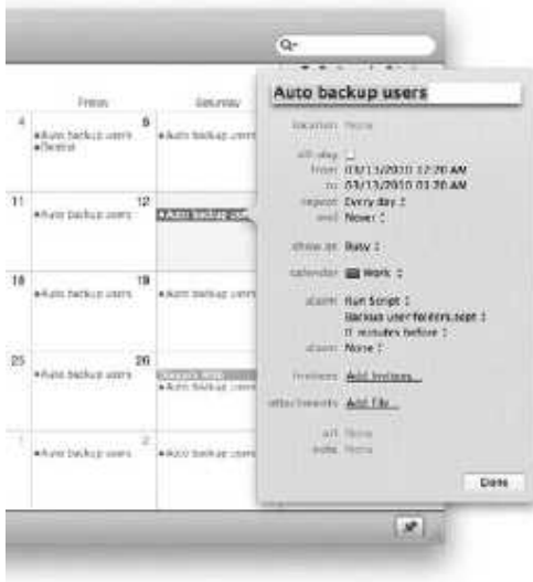
Figure 23–4. The event shown will run the Backup user folders.scpt script every night at 12:20 AM.
