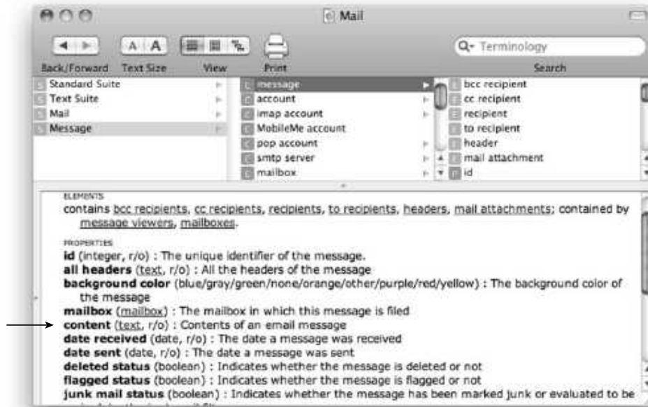
Figure 7-14. Part of the Mail application's dictionary, showing the content property defined by the message class
