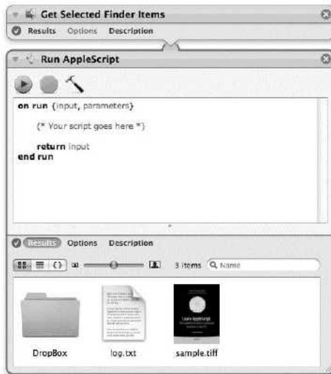
Figure 21–10. The workflow containing the two actions and the Run AppleScript's action result
