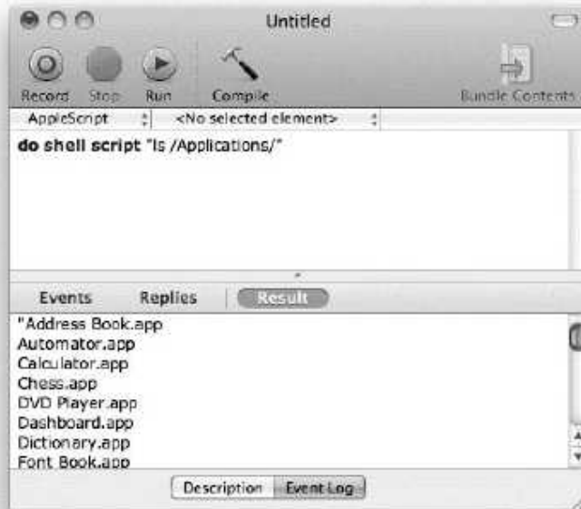
Figure 27–2. Running the ls Unix command from AppleScript using the do shell script command
