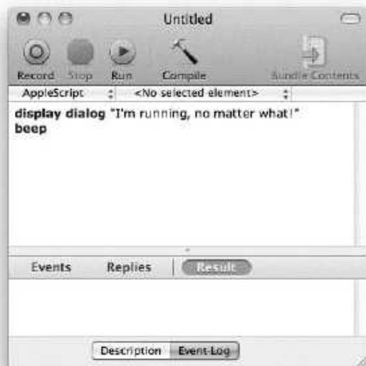
Figure 18–2. The script has a run handler, but it is implied. The entire script shown is part of this run handler.
