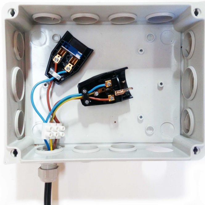
Repeat the wiring for the non-grounding connector with the remaining brown and blue leads.
