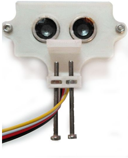
A 3D printed Ultrasonic Ranger case
