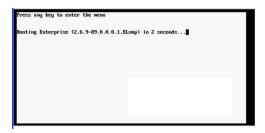
5. A screen similar to the one shown below appears on the attached monitor. Use the mouse or arrow keys to select **System Restore** and press **Enter**. The HPE System Restore utility launches.
