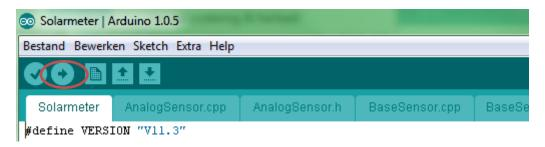
When uploading is finished, you can disconnect the board, put it in your meter cabinet and power up.
