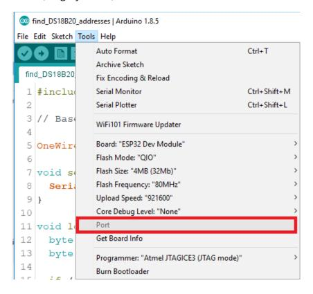
It might be one of these two problems: **1. USB drivers missing** or **2. USB cable without** data wires.
