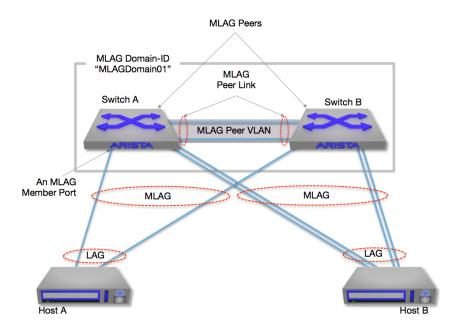
Figure 5: Arista Multi-Chassis Link Aggregation Architecture
