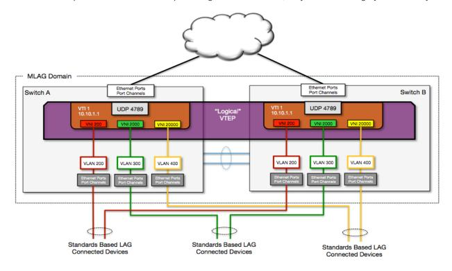
Figure 7: Arista VXLAN+MLAG Hardware VTEP Architecture
