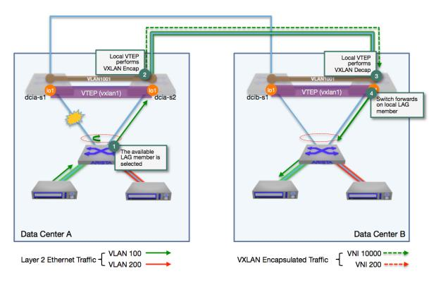
Figure 15: Effect of Local MLAG Member Port Failure
