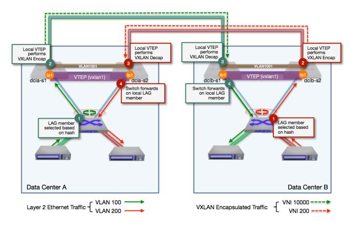
Figure 14: Normal VXLAN+MLAG forwarding Mechanism
