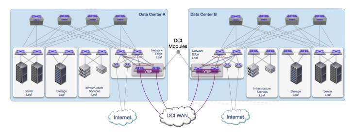
Figure 9: Integration of the DCI module with a Leaf-Spine Data Center Network
