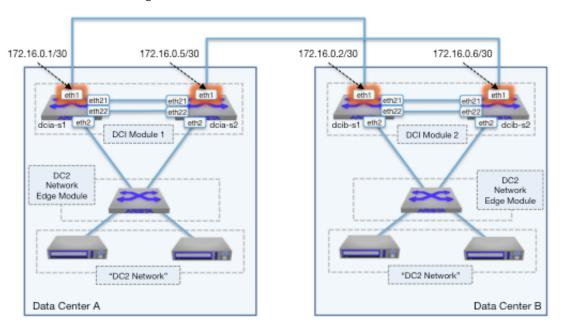
Figure 11: Example DCI Solution - Layer-3 Interfaces
