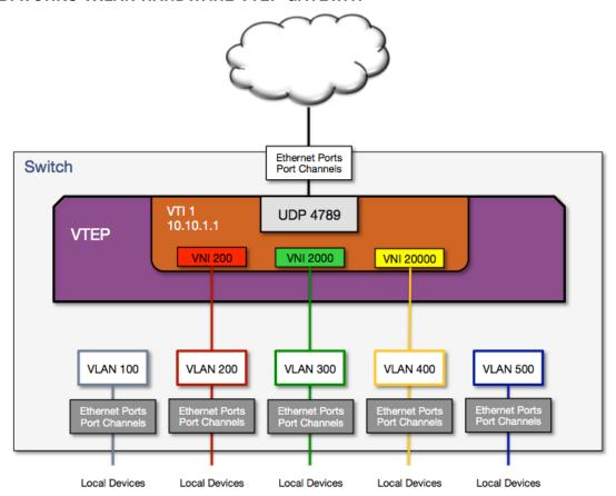
Figure 3: Arista Hardware VXLAN Gateway Architecture
