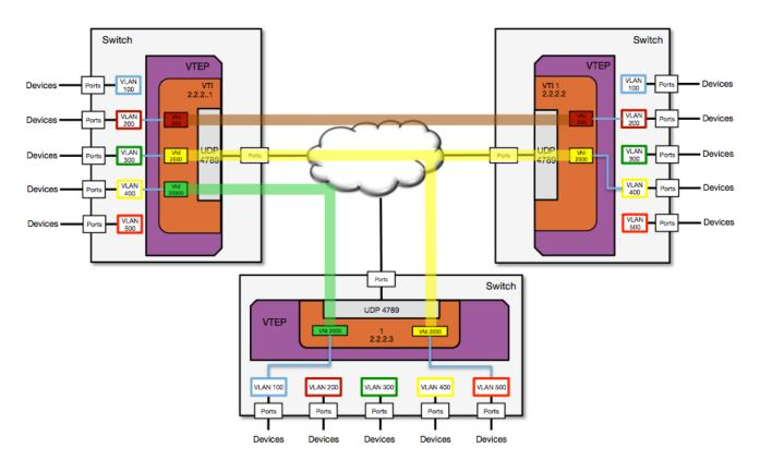
Figure 4: Arista VXLAN Point-to-Point & Multipoint VNIs with VLAN Translation
