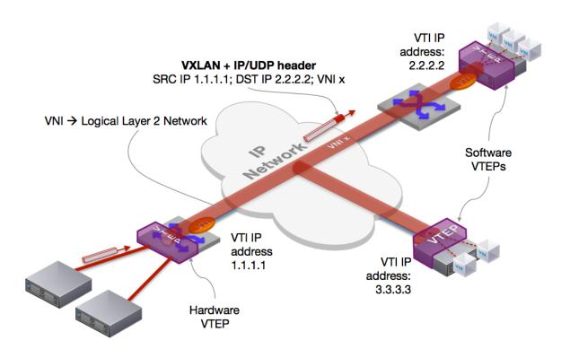
Figure 2: VXLAN Components and Operation
