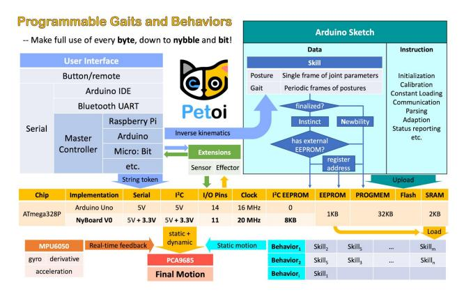
One frame of joint angles defines a static posture, while a series of frames defines a periodic motion, usually a gait.
