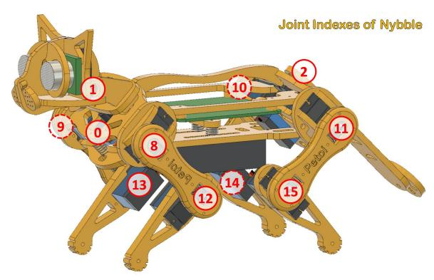
Use h for head, t for tail, r for shoulder roll joint, s for shoulder pitch joint, k for knee joint, F for front, H for hind, L for left, R for right, the full joints map of OpenCat is:
