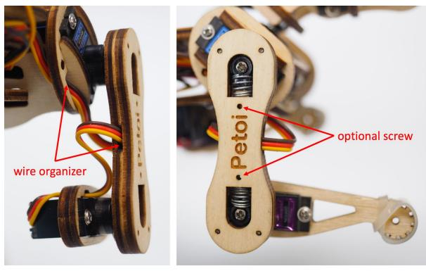
The servo arm should be able to slide in the track on thigh2 with subtle friction after thigh1 and thigh2 are screwed together. You can tune the tightness of screw C to achieve proper friction. If you need more control on the tightness:
