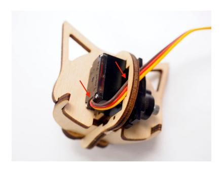
3.1.5. DO NOT connect the head with neck yet, because the tilt servo on the head has to be calibrated.
