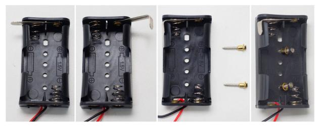
The spring attached structure of the battery holder is used for shifting the center of mass when fine tuning gaits.
