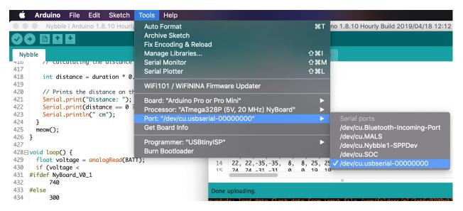
If Tx and Rx keep litting up, there's something wrong with the USB communication. You won't see the new port. It's usually caused by overcurrent protection by your computer, if you're not connecting NyBoard with external power supply and the servos move all at once.
