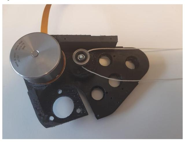
Step 12: The process of readying the gear spindle and motor spindle is repeated, and the motor spindle and gear
