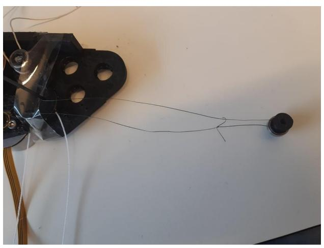
$Step\ 15:$  Mount the gear top, and tighten the string by twisting it around. Then lock it in place by inserting the hex nut and tightening the bolt.
