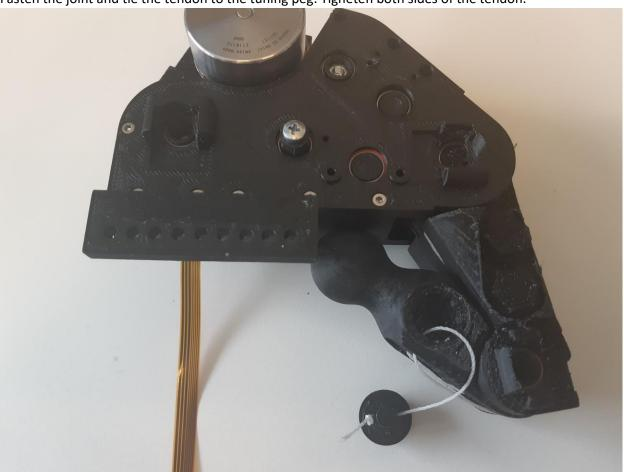
Step 28: Insert magnets into the cup of the motor spindles, and joints.
