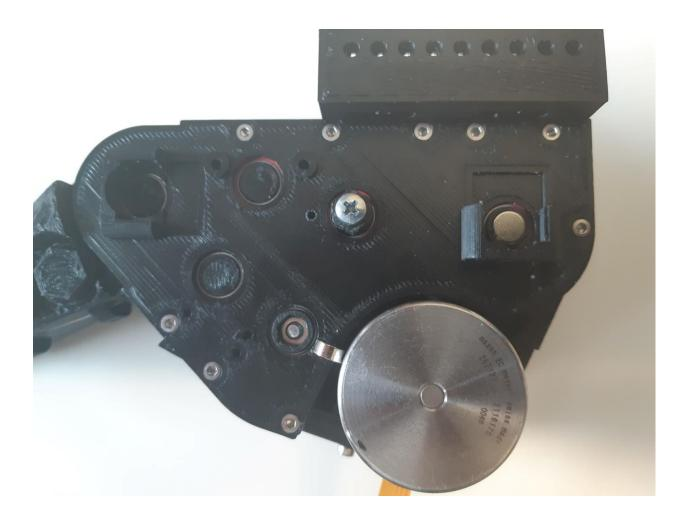
Step 29: Slide sensors into sensor slots and attach the cables. Cable clamps can be mounted anywhere to route the cables as you see fit.
