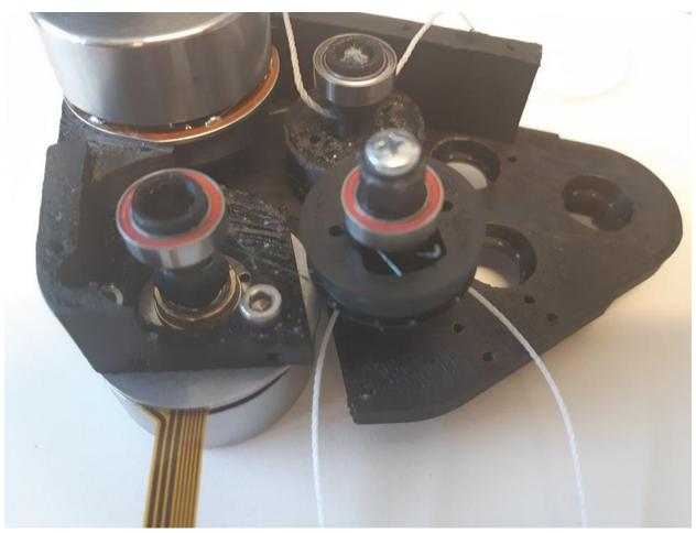
Step 16: With both the backplate and front plate in place; move the motor back and forth and try to make the string between the gear spindle and motor spindly into a nice and tidy spiral. Tighten any slack.
