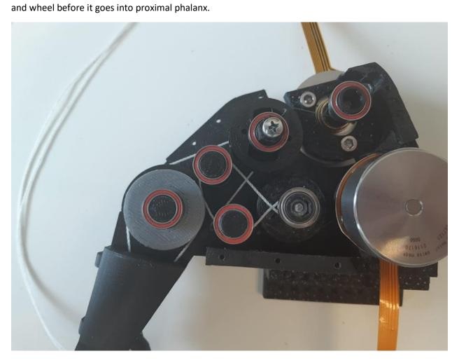
Step 26: From the wheel, to the MCP joint, the tendon is in crossed configuration. Route them around the last pulley and into the tightening slot
