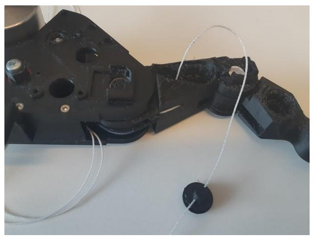
Step 21: Rotate the tuning peg to tighten the string and insert it into the slot.
