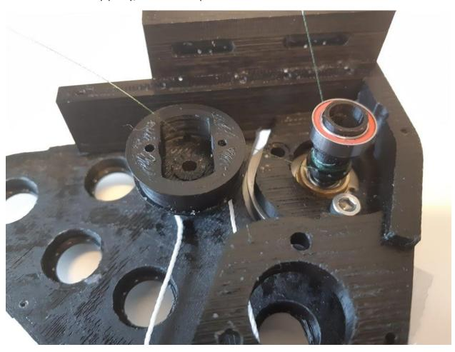
$Step \ 8$  The other side of the string goes directly from the motor spindle and is wound around the gear spindle until it is of the same length as the string that is already in place
