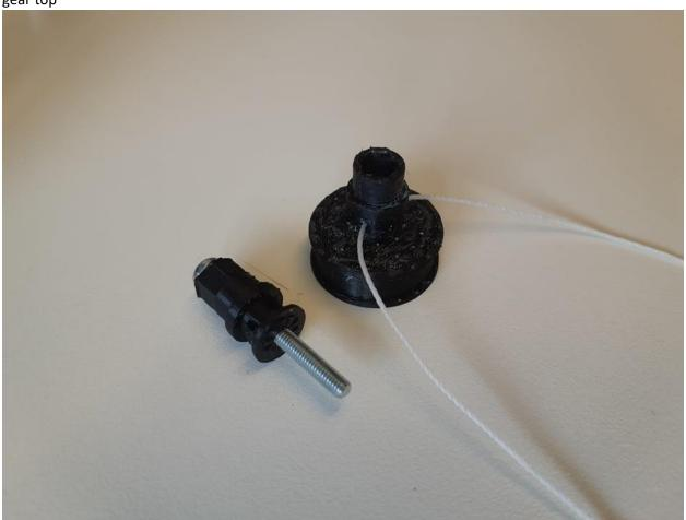
Step 4: Use the bolt to push the string out of the hole in the middle of the gearspindle. The string will later be locked in place when the hex nut is placed at the end of the bolt.
