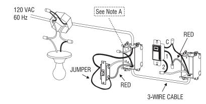
The "common" wire, previously identified upon removal of the old switch, must be connected to the "C" wire of the programmable wall switch. Connect the two other wall switch wires to the two remaining wires (see above).
