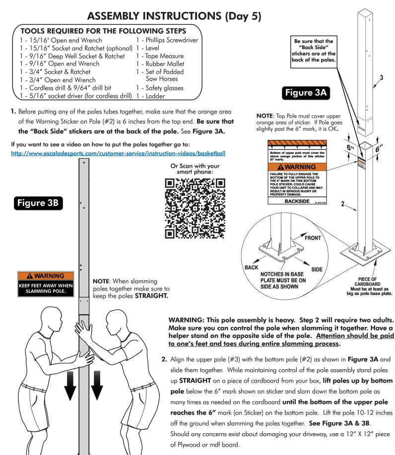
**NOTE:** When Slamming the pole together make sure you place the cardboard on a **flat surface** like concrete or Asphalt, do not slam pole on grass or soft ground.
