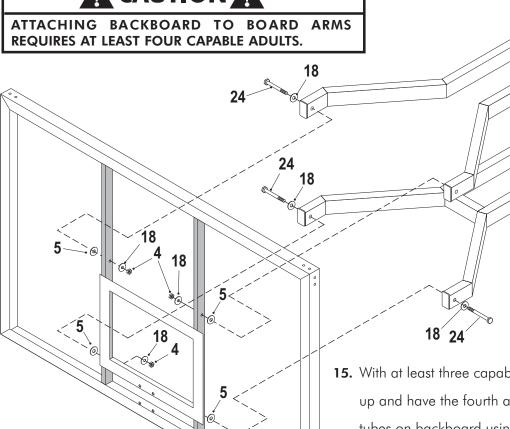
15. With at least three capable people, raise the backboard assembly up and have the fourth attach Lower Board Arms to lower mounting tubes on backboard using two bolts (#24), two plastic washers (#5), four washers (#18) and two lock nuts (#4). See **Figure 12**.
