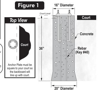
Note: Using a concrete form for the top 4" of the concrete is recommended. Cardboard forms can be purchased at some hardware and home stores or a wooden form can be constructed out of 2 x 4's.
