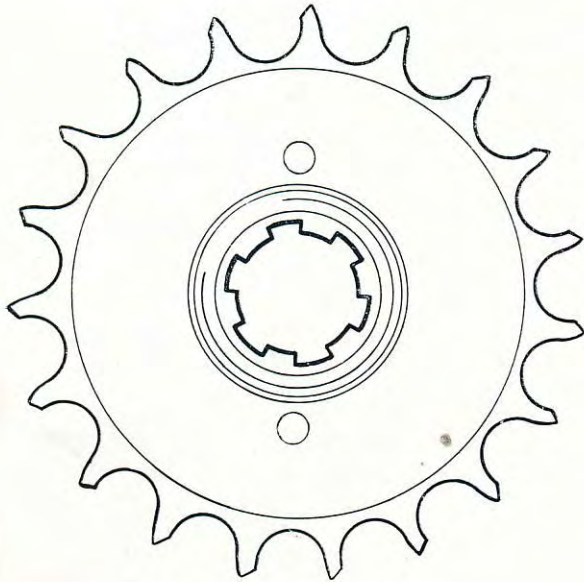
FIG. H4. Worn sprocket.
