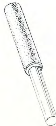
FIG. K5. 61-3382 Valve guide fitting and extracting punch.
