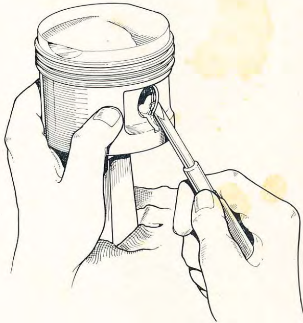
FIG. B7. Removing circlip.
