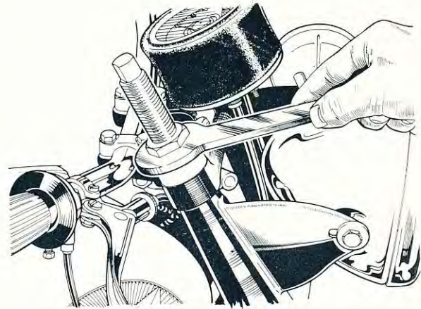
FIG. E11. Using service tool No. 61-3824 to reassemble the forks.
