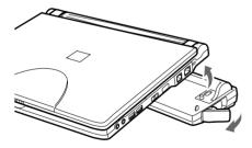
Figure 4-13 Removing the Port Replicator
