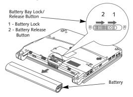
Figure 4-1 Removing the Battery
