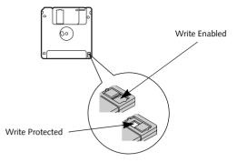
Figure 4-5 Floppy Disk Write Protect
