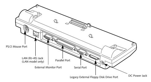
Figure 4-9 Port Replicator rear panel (LAN model shown)
