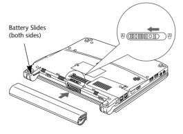
Figure 4-2 Installing the Battery
