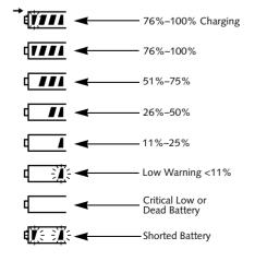
Figure 2-10 Battery Level Indicator
