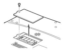
Figure 4-6 Opening the Memory Upgrade Compartment
