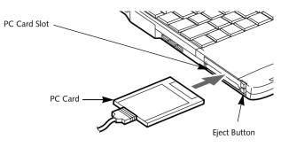
Figure 4-5 Installing/Removing PC Cards
