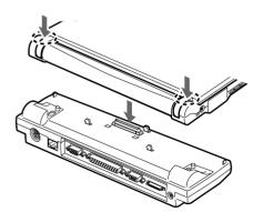
Figure 4-11 Attaching the Port Replicator
