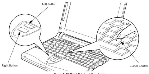
Figure 2-12 Quick Point pointing device
