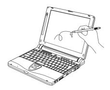
Figure 2-16 Using the Stylus with the Touch Screen
