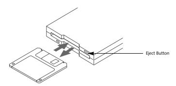
Figure 4-3 Loading/Ejecting a 3.5" Floppy Disk
