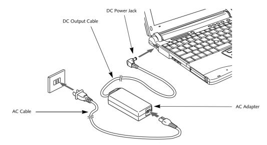
Figure 3-1 Connecting the AC Adapter
