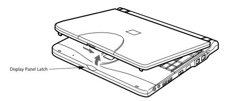
Figure 3-2 Opening the Display Panel
