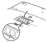
Figure 4-7 Installing a Memory Upgrade Module
