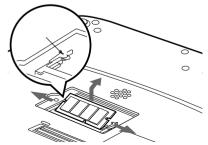
Figure 4-8 Removing a Memory Upgrade Module
