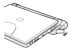
Figure 4-12 Unlatching the Port Replicator
