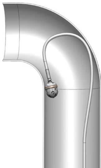
IMPROPER USE: Badger will turn around in large diameter pipe VERY DANGEROUS!
