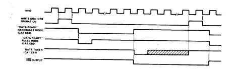
Figure 22.5 – Write Handshake Timing
