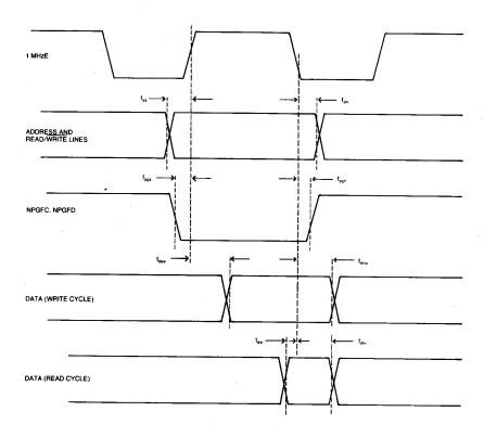
Figure 28.5 - 1MHz bus timing
