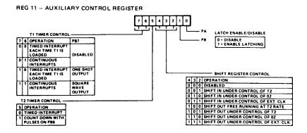
Figure 22.10 – Auxiliary Control Register
