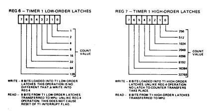
Figure 22.8 – T1 Latch Registers
