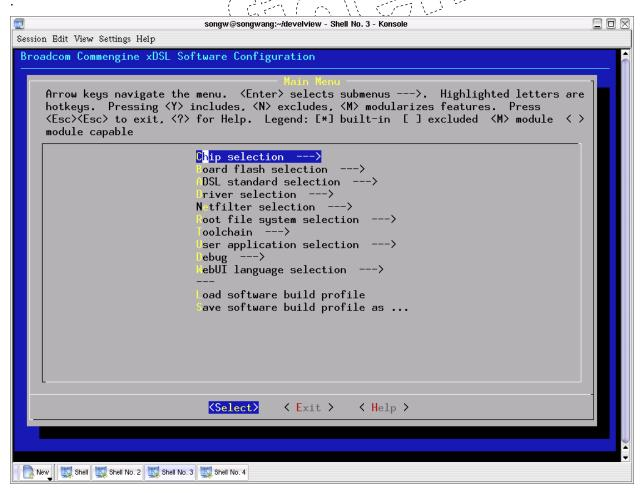
By selecting "Load software build profile", you can load an existing profile, such as 96345GW or 96345R, and then you can modify configurations and select "Save software build profile as..." to create your own platform build profile. You can also start from scratch to create a profile. Following steps show how to create a customized profile based upon 96345GW profile.
