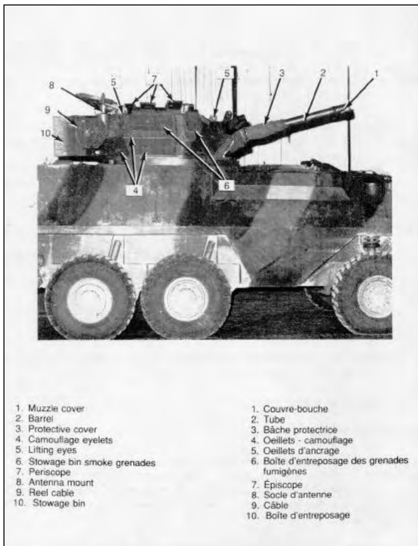
Figure 1-2-1 Turret Side View (Right-Hand Side)
