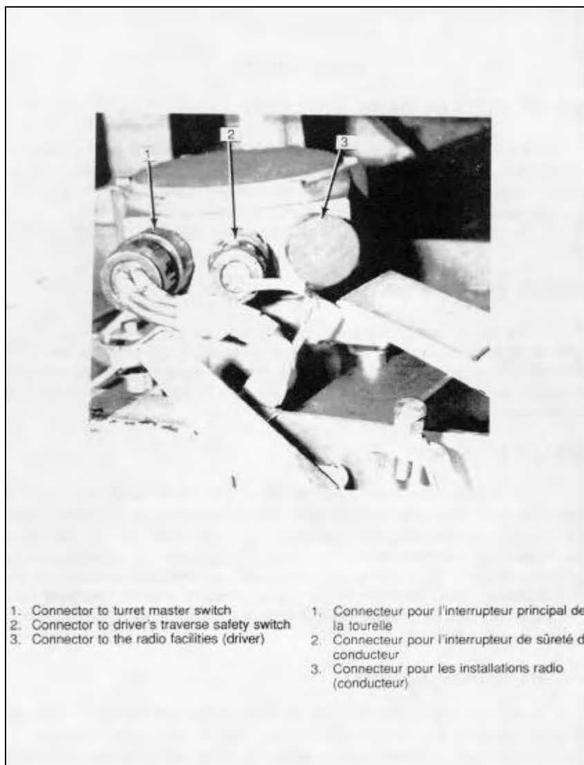
Figure 4-2-1 Turret Rotary Base Junction
