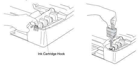
3 Open the new ink cartridge bag for the colour shown on the LCD, and then take out the ink cartridge.
