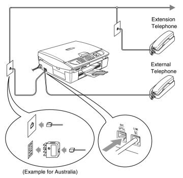
When you are using an external or an extension, the LCD shows Telephone.
