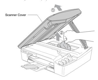
If the paper is jammed underneath the print head, disconnect the machine from the power source so you can move the print head to take out the paper. **5** Lift the scanner cover to release the lock. Gently push the scanner cover support down and close the scanner cover.
