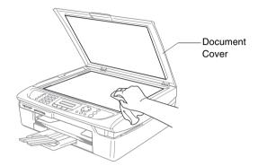
Clean the glass strip under the film with isopropyl alcohol on a lint-free cloth.
