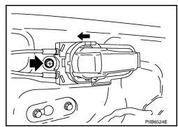
Disengage the handle from the door panel, and remove the inside handle.
