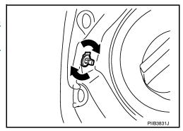
5. Remove fuel filler lid opener cable clip from the vehicle.
