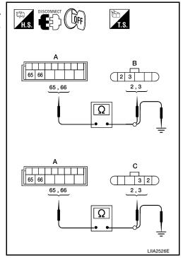
Check continuity between BCM connector (A) M20 terminals 65, 66 and body ground.
