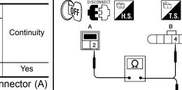
Check continuity between trunk lid opener switch connector (A) B128 terminal 2 and ground.
