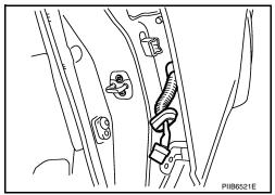
3. Remove the check link bolt.
