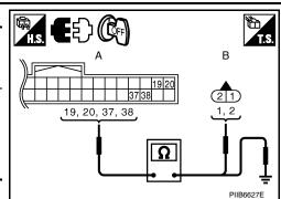
Check continuity between Intelligent Key unit connector and ground.
