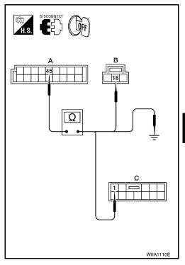
4. Check continuity between BCM connector M19 (A) terminal 46 and main power window and door lock/ unlock switch LH connector D7 (B) terminal 6 or power window and door lock/unlock switch RH connector D105 (C) terminal 2.
