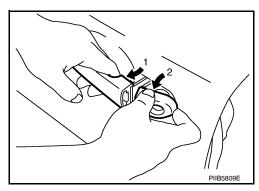
13. Pull the outside door handle forward and then slide it toward the rear of the vehicle to remove.
