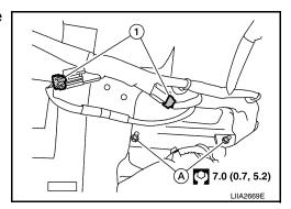
3. Release the clips and remove the switch from the housing.
