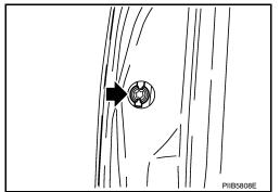
12. Remove the door cylinder assembly while pulling the outside handle forward.
