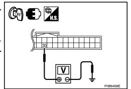
Check Back Door Opener Switch Circuit (Without Intelligent Key, with Power Windows)
