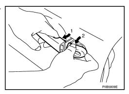
7. Pull outside door handle forward (1), and slide it toward the rear of the vehicle to remove (2).
