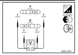
3. Check voltage between rear door lock actuator connector LH (A) D205 or rear door lock actuator connector RH (B) D305 terminals 2 and 3.
