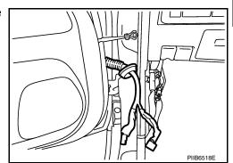
Remove the check link bolt.
