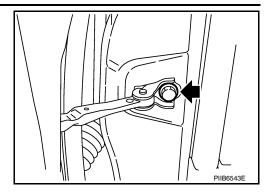
4. Remove the hinge nuts and the door assembly.
