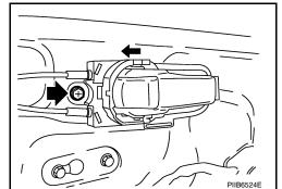
4. Disconnect the inside handle and lock knob cables from the inside handle.
