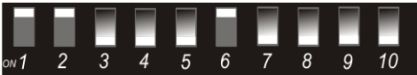
DIP switch setting (default) for high volume, audio player active, alarm zone 1, radio channel 0
