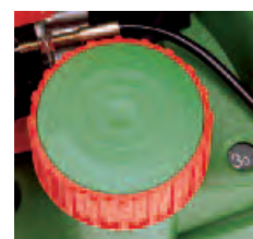
The height adjustment is central and can be continuously adjusted from 30 to 80 mm.
