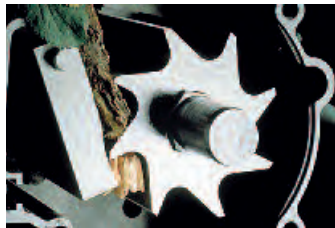
With the LH and ESK shredder, the cut material is drawn in by the rotating cutting wheel.
