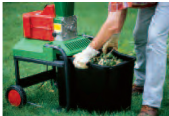
The 64 l collector box protects the blade access from below.
