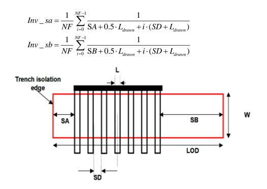
Figure 14.3 Layout of multiple finger MOSFET
