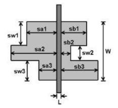
Figure 14.4 A typical layout of MOS devices with more instance parameters (swi, sai and sbi) in addition to the traditional L and W
