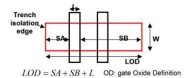
Figure 14.1 shows the typical layout of a MOSFET
