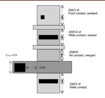
Figure 12.1 Definition for layout parameters.
