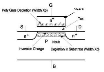
Figure 1.2. Charge distribution in a MOSFET with the poly gate depletion effect. The device is in the strong inversion region.
