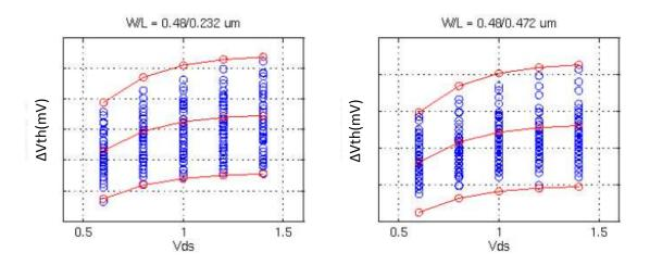
Figure 2.1 Asymmetric dependence of  $V_{th}$  variation on  $V_{ds}$
