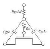
In this case, the gate electrode resistance given by (9.10) is in series with the intrinsic-input resistance  $R_{ii}$  as given by (9.6) through two internal gate nodes, so that the overlap capacitance current will not pass through the intrinsic-input resistance. *trnqsMod* = 0 (default) and *acnqsMod* = 0 (default) should be selected for this case.
