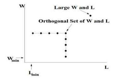
Figure 16.1 Device geometries used for parameter extraction
