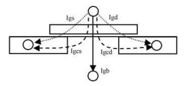
Figure 4.1. Shematic gate current components flowing between nMOSFET terminals in version.
