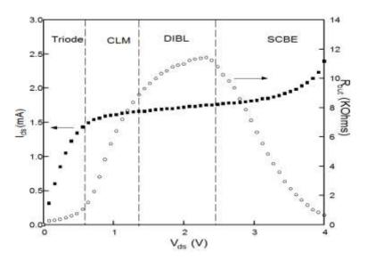
Figure 5.1 General behavior of MOSFET output resistance.
