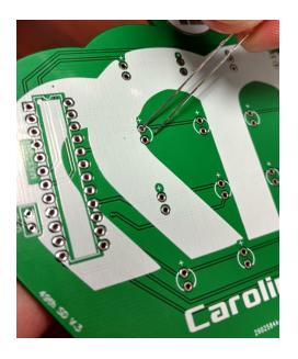
Insert the 16 LEDs into the front of the PCB. Ensure the longer lead goes into the hole with the "+" label.
