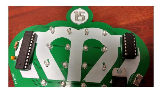
Place the ATTINY84 into its socket and the MAX7219 into its socket. Ensure the round notch is facing upwards Congratulations! The badge is finished!
