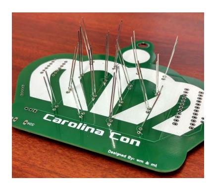
Now that the PCB is upside down you may solder the LEDs to the PCB. Try and keep the leads as straight in the air as possible.
