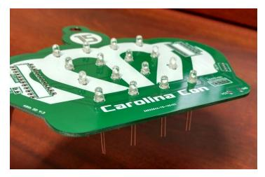
Once the LEDs are in place carefully flip the PCB upside down so that the leads are sticking up.
