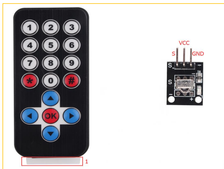
Figure 3.2.5.1 Physical Map of Remote Control Suite
