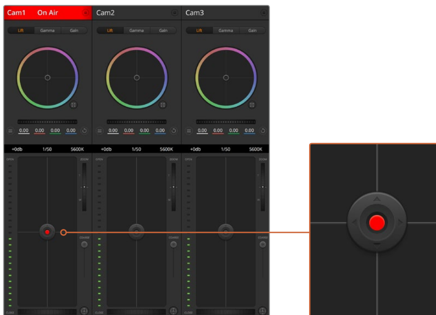
The iris/pedestal control illuminates red when its respective camera is on air
