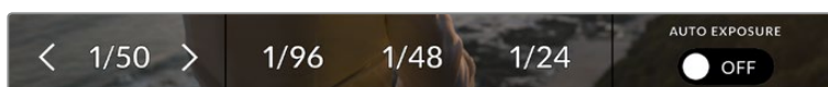
Your URSA Broadcast will suggest flicker free shutter speeds based on the mains power frequency you choose in the 'setup' menu
