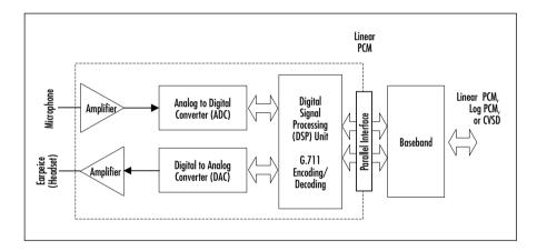
Figure 9.1 General Block Diagram of Bluetooth Codec
