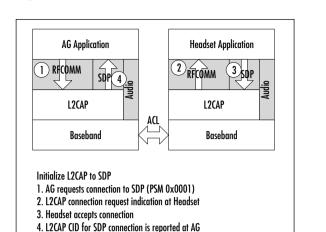
Figure 2.5 Simplified L2CAP Connection to SDP Procedure
