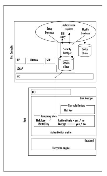
Internal to the Security Manager is a service database, a repository that is configured by the user via application software. As will be explained later, this database is used to implement Mode 2 security and is referenced by the Security Manager to determine which security measures to invoke and when to invoke them. In addition to this, there is a device database which stores link key information, and also keeps tabs on which devices are Trusted and which are not.
