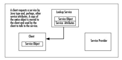
Figure 5.5 Using a Service in Jini
