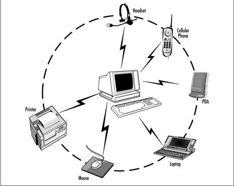
This fully wireless scenario can be achieved because of the master/slave nature of the Bluetooth technology. All devices are peers, identified by their own unique 48-bit address, and can be assigned as a *master* either by function or user intervention. A master can connect to up to seven *slaves* at the same time, forming a *piconet*—this "point-to-multipoint" feature is what sets Bluetooth apart from other wireless technologies. Figure 1.2 illustrates several connection scenarios.
