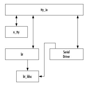
Figure 6.2 Stacked TTY Driver Configuration
