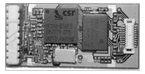
The PCB issues examined in the previous method are irrelevant when using a module since we just solder the module onto our own PCB. There are no new Bluetooth technology-induced RF layout considerations or BGA placement issues. Of course, we must ensure that the antenna is placed in a position where propagation is not adversely affected by surrounding components, and this will require some RF expertise. But antenna siting is really the only RF issue we have to think about.
