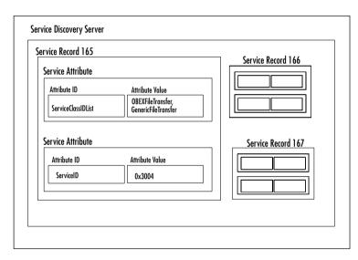
Figure 5.2 The Data Structures of a Sample SDP Server
