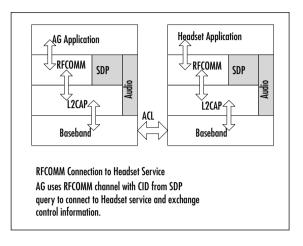
Figure 2.8 Simplified L2CAP Connection to RFCOMM Procedure
