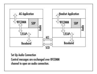
Once the user has accepted the call, a voice (SCO) link must be set up (see Figure 2.10). Although this link is controlled using the RFCOMM link, it is established separately, usually by a separate audio control layer. Once the SCO link is established, it is still controlled by the RFCOMM link. For instance, some headsets support remote volume control using AT commands, and the
