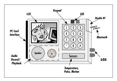
A keypad is useful to answer any questions or enter PIN codes to authorize access to the device, and to control more complex functions on the device. If the PIB does not have a keypad, it would have to use a pre-programmed fixed PIN code, which prevents the user from easily changing the code if they want to bar somebody who was previously granted access to data.
