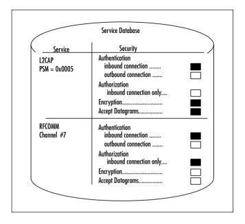
Figure 4.4 The Service Database Determines When to Invoke Security
