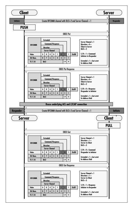
Figure 10.12 Format of OBEX Messages between Client and Server
