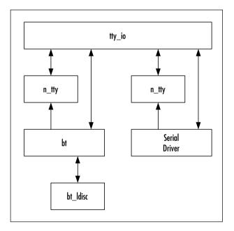
Guess what? That's exactly how we make the Bluetooth driver talk to a Bluetooth card attached by a serial cable. Figure 6.2 shows a picture of this. The  $bt\_ldisc$  in effect will route all data to and from the serial port through the Bluetooth driver. That's where all the parsing and packet assembly will take place.
