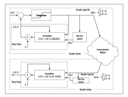
Figure 9.5 The CVSD Encoder and Decoder Block Diagram
