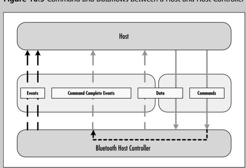
Figure 10.9 Command and Dataflows between a Host and Host Controller
