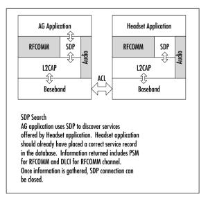
The Audio Gateway will send requests to retrieve the service record for the Headset Service. This checks that the service is really supported, and provides information on how to connect with it.
