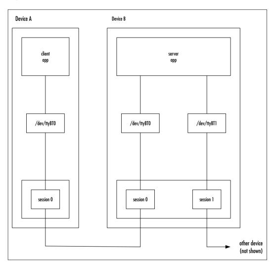
Figure 6.4 Multiple Simultaneous RFCOMM Connections
