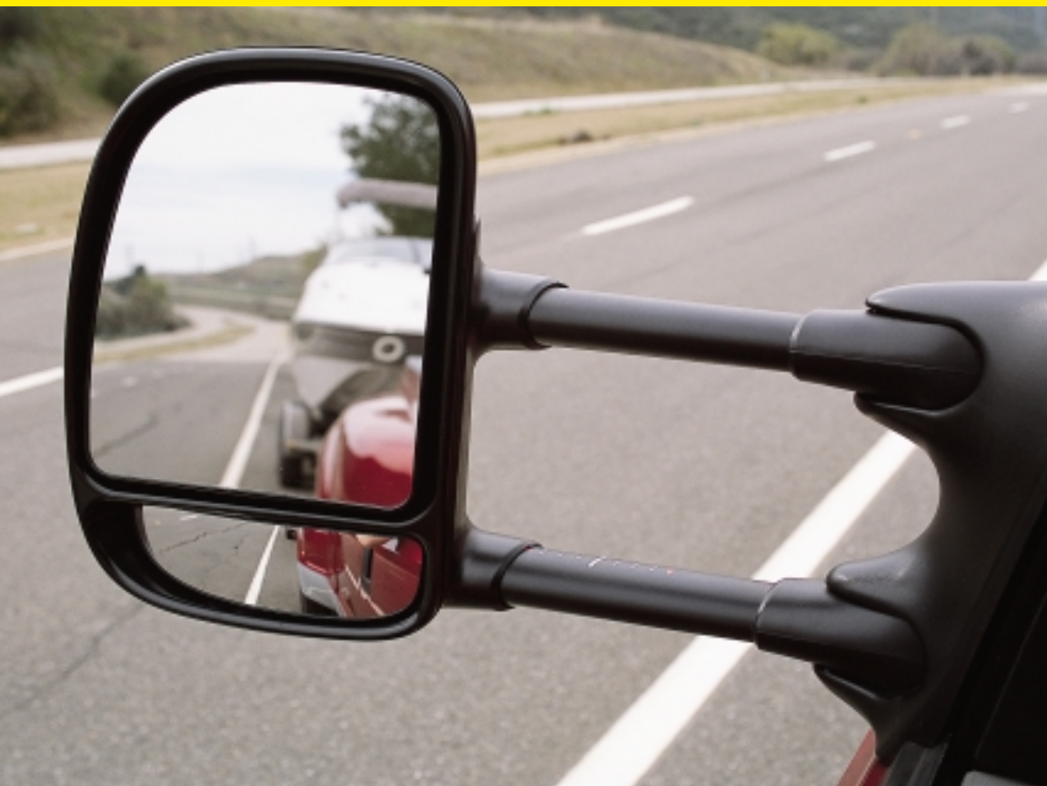
EXTENDED SIDE-VIEW MIRRORS are especially useful when towing large boats or camping trailers.
